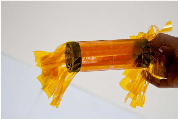
Figure 4: Prototype of the inner detector layers built from Kapton® foil and thin glass plates representing the HV-MAPS sensors.
