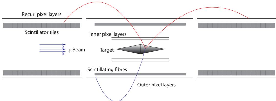
**FIGURE 3.** Schematic view of the Mu3e detector
