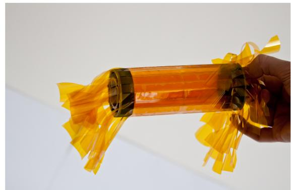
**FIGURE 4.** Mechanical support structure for the vertex tracker
