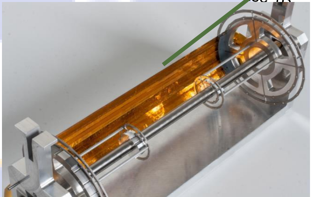
Layer 3 early prototype in assembly frame with 50µm glass "chips"
