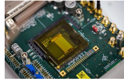
MuPix8 on test board
