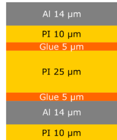
Foreseen lay-up of aluminium kapton flex circuit (LTU)
