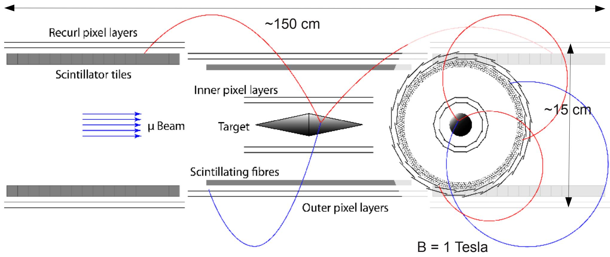
Geometrical acceptance **~70 %** for  $\mu^+ \rightarrow e^+ e^+ e^-$  decay
