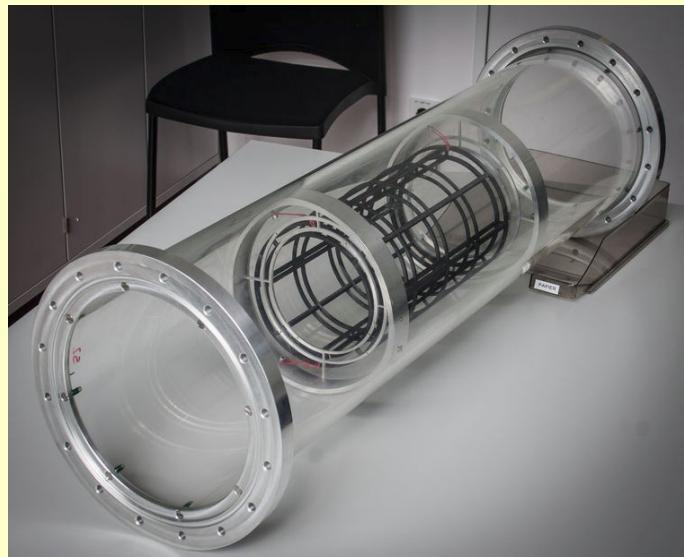
Cooling flow reactor for tests
