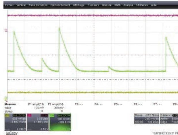
The chip works, particles are measured when the chip is in the beam: Output of the amplifier
