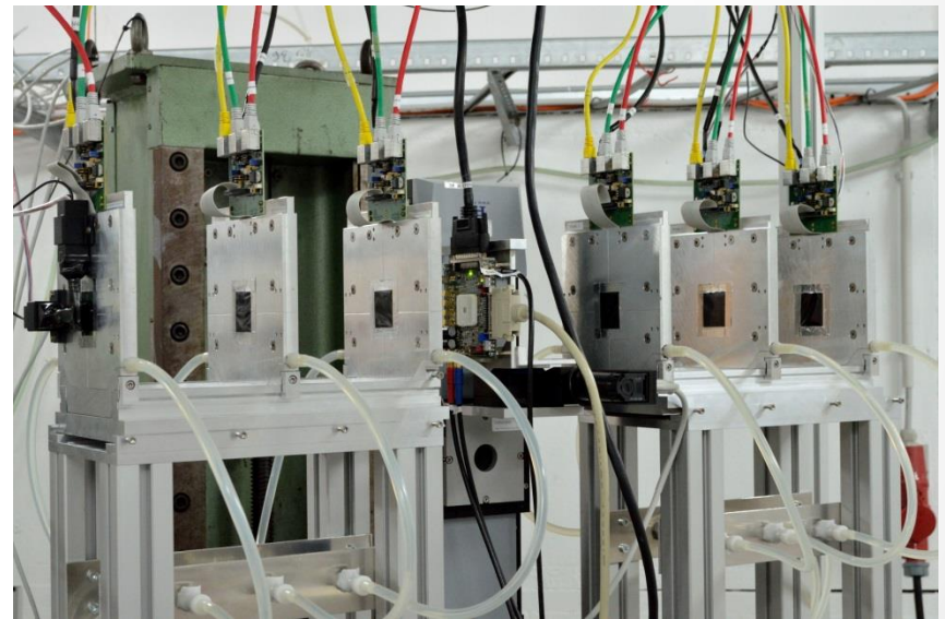
MuPix7 @ DESY test-beam in EUDET telescope
