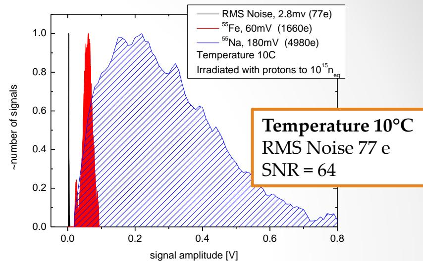
$^{55}\text{Fe}$  and  $^{22}\text{Na}$  spectrum, RMS noise
