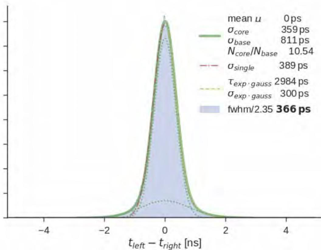
Timing resolution  $< 400\text{ ps}$  including ASIC (using a  $\text{Sr}^{90}$  source)
