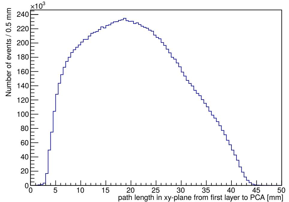
$$\left. \begin{aligned} \sigma_{MS,PCA} &= \sigma_{MS,first\ layer} \cdot s \approx 0.8\ mm \\ \sigma_{pixel} &= 0.08\ mm / \sqrt{12} = 0.02\ mm \end{aligned} \right\}$$
