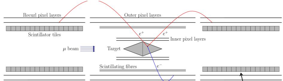
Particles (electrons) bend back in magnetic field:
