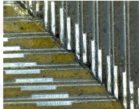
Test structure for wire bonding on flexprints
