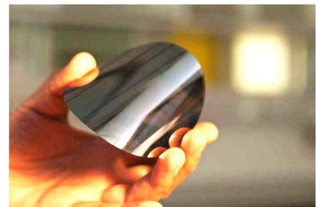
50 µm thin silicon wafer
