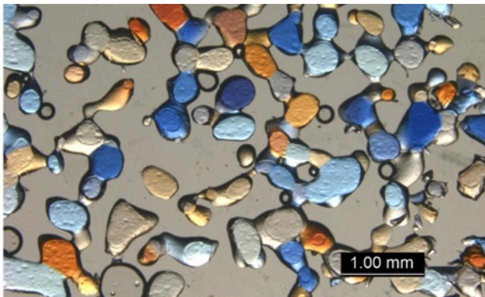
Figure 5.8: Grain boundaries of natural snow made visible with the cross polarizer technique from Riche et al. (2012b).
