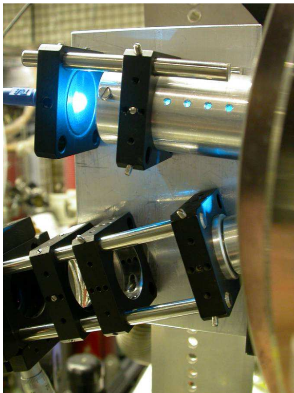
Figure 3.7: The Ar laser light is coupled to the laser head via optical fiber. The simple but stable and easily adjusted setup of the laser head (upper) and Raman collector (lower) is displayed.
