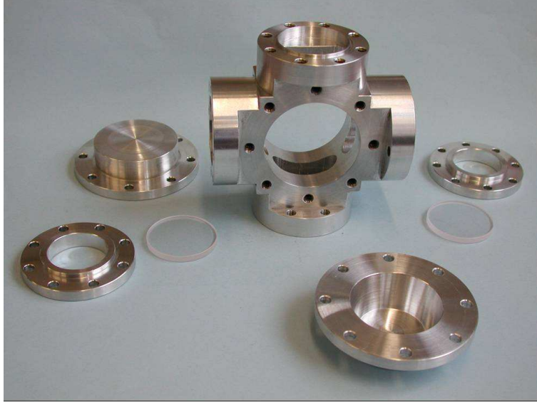
Figure 3.1: The major mechanical pieces of the cryogenic target cell are displayed: The cell body, the reentrant neutron beam windows, the optical sapphire windows with Al press rings. The vertical axis of the cell is for cooling (from below) and gas connections (from above) as well as thermometry and heating. All flange connections are sealed with indium.
