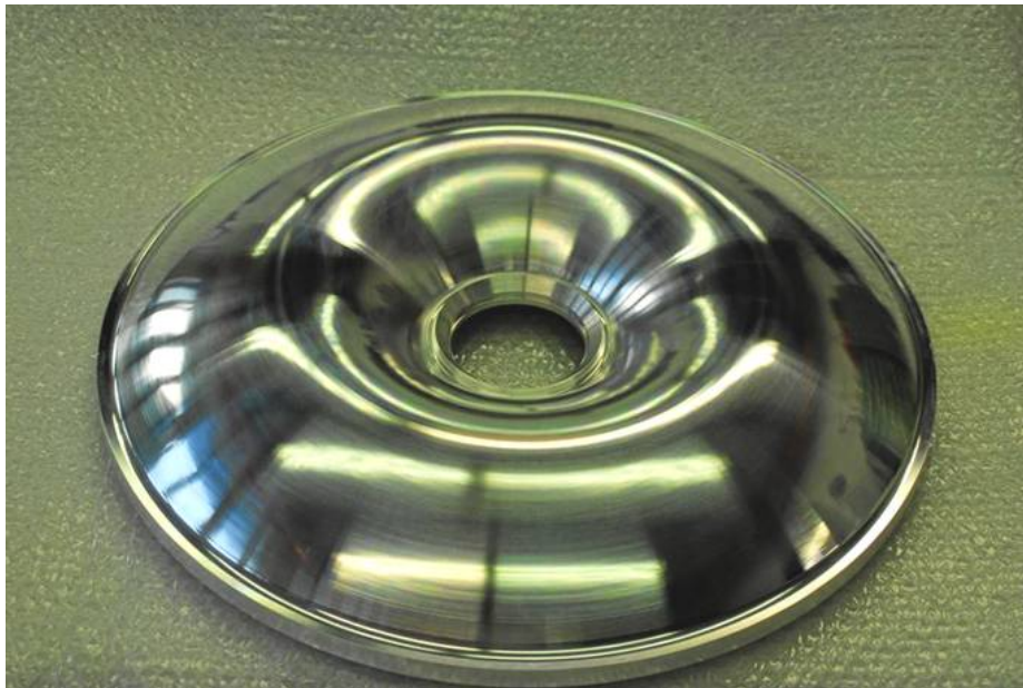
Figure 2.10: The toroidal shaped sD 2 converter lid made from AlMg3.
