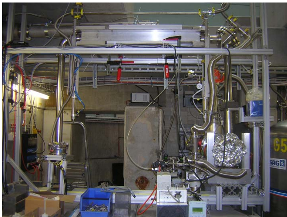
Figure 4.13: The Storage bottle mounted in the UCN detection system.
