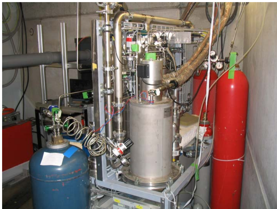
Figure 4.9: Rear view of the gas system. In the middle one can see the ortho/para converter.
