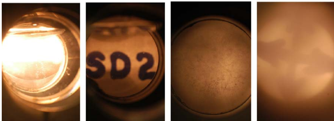
Figure 4.21: The comparison of the transparencies of a crystal grown from the liquid (at 18K, two pictures on the left) and grown from the gas phase (at 12K, two pictures on the right).
