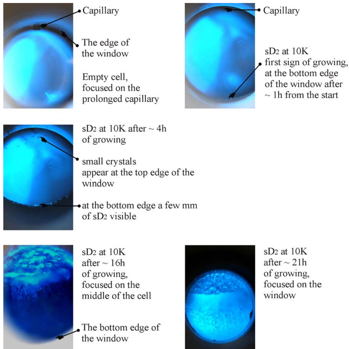
Figure 4.18: The process of growing the crystal from the gas phase is shown and described.
