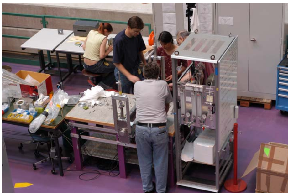
Figure 4.12: Building the AI support for the storage bottle and connecting the shutters.
