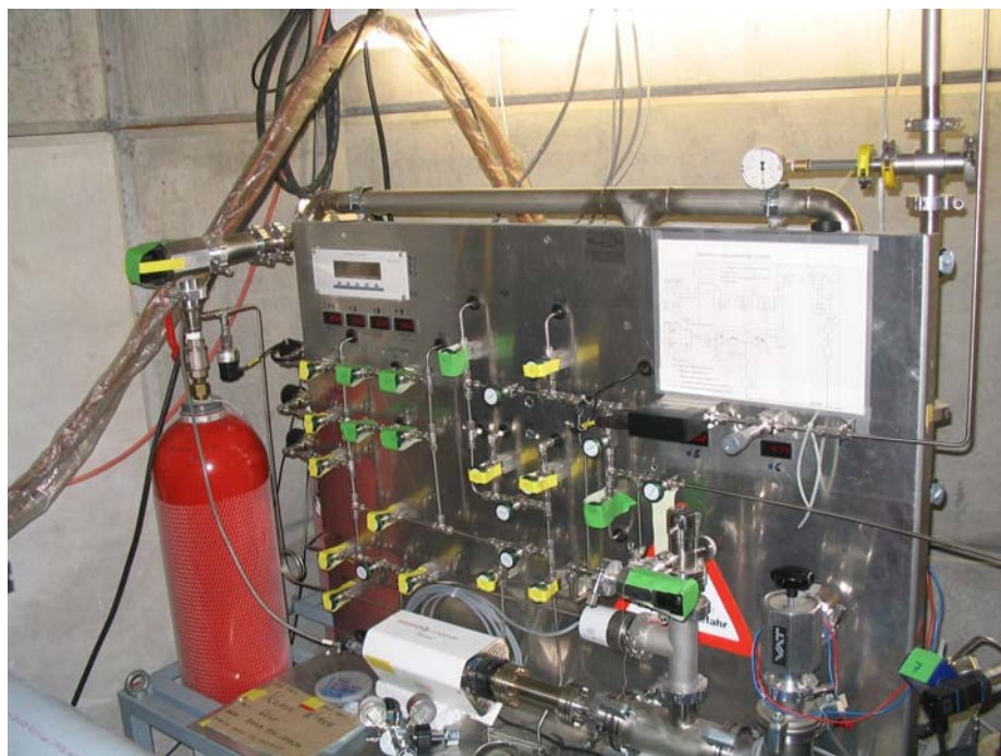
Figure 4.8: Front view of the gas system of the UCN production experiment.
