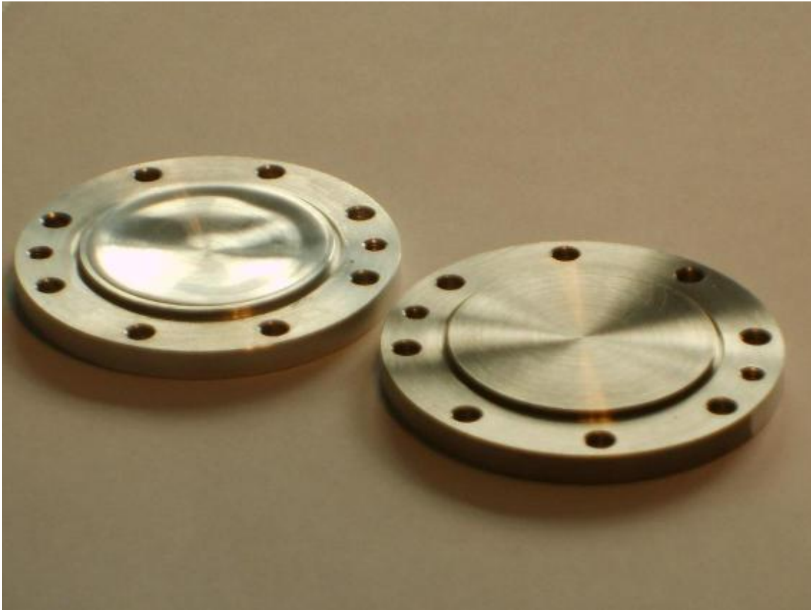
Figure B.9: An alteration of the shape of the neutron window by pressure. The new window is shown on the right, the deformed one on the left.
