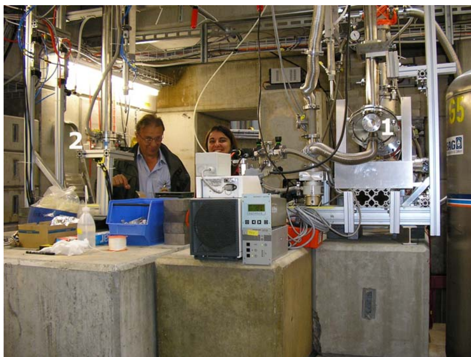
Figure 4.17: The mounted flange with the beam dump and an Al vacuum window through which CN pass to enter the TOF system (1) and the UCN detector placed on the Al support (2).
