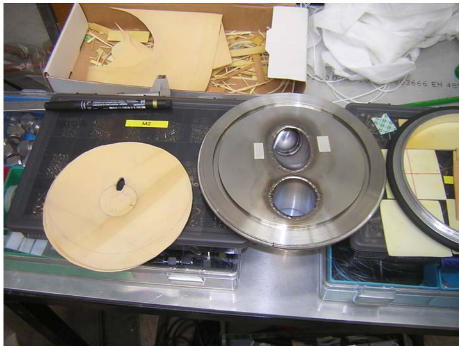
Figure 4.14: The beam dump made of {}^6\text{LiF} with a hole and an Al flange used for mounting the beam dump.
