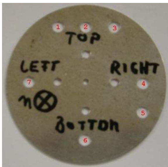
Figure 3.11: The cadmium mask that is used to determine the position of the signal on the detector.
