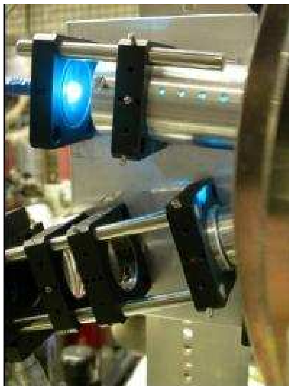
Figure 3.8: The Raman head consists of the laser head (upper) for the light input and Raman collector (lower) for the scattered light. The Ar laser light is coupled to the laser head via optical fiber.
