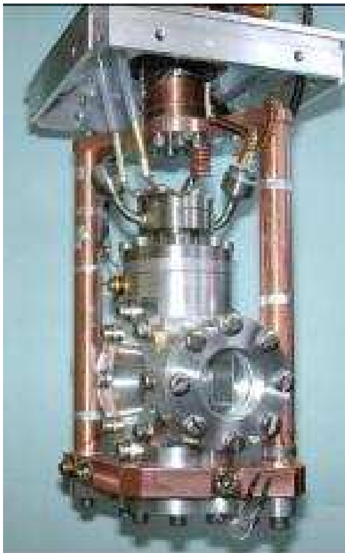
Figure 3.4: The sD_2 cell mounted on the cryostat
