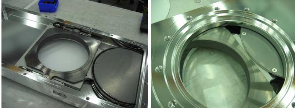
(a) Shutter disc (right) and expanding rings for slit reduction in the open position (left).
