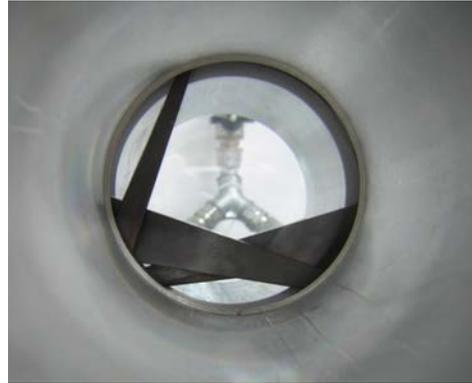
(b) The beam line partially covered by plexiglass discs, the very bottom of the beam is open, the upper part is covered.
