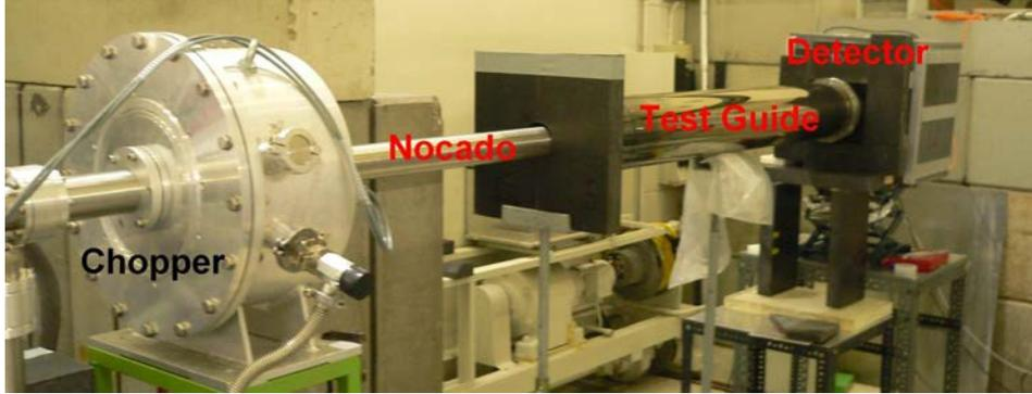
Figure 4.3: Setup for the transmission experiment made in Mainz, April 2008.
