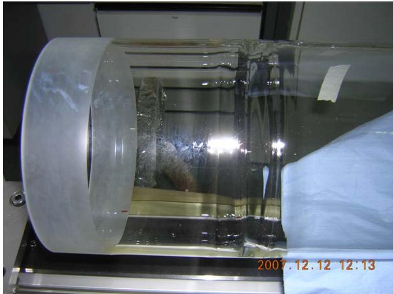
Figure 3.1: The machined glass end piece joined to a glass tube inside the furnace.
