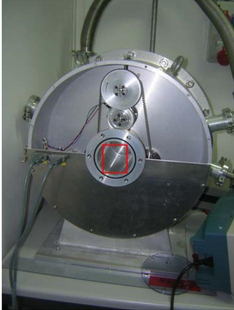
(a) Front view of the neutron chopper, the top cover is taken off, so one can see the axes of the plexiglass discs. Picture (b) shows a zoom into the beam line (red square)
