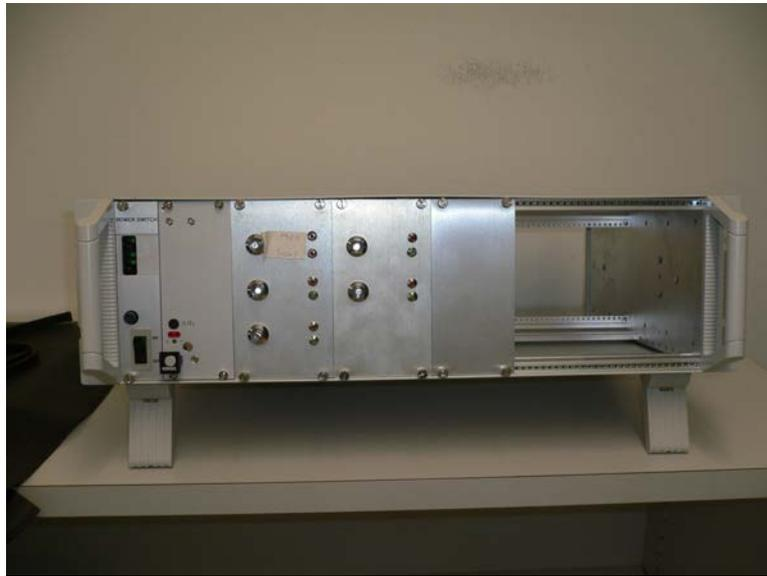
Figure 3.6: The control box, components from left to right: the power switch with the mounted 5 V power supply, the 24 V power supply, the master board, the slave board and finally the National Instruments board.
