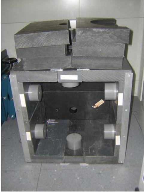
Figure 3.16: Shielding for the Cascade-U detector. The front parts are placed on top of the box.
