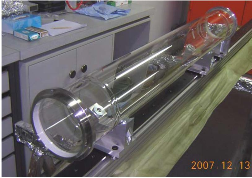
(a) Uncoated guide with flanges glued on the ends.
