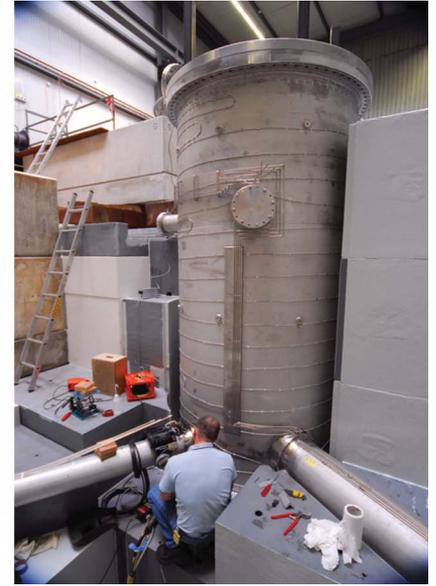
**Figure 4.** a) Schematic view of the main components of the ultracold neutron source at PSI contained in a large moderator and vacuum tank system. b) Picture of the UCN vacuum tank taken during construction in spring 2009, showing the main neutron guides’ vacuum tubes being prepared for welding.
