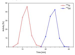
**Fig. 1:** Elution profile of the separation. The impurities <sup>133m</sup>Ce, <sup>133</sup>Ce, <sup>133</sup>La and stable zinc remain on the column during elution.
