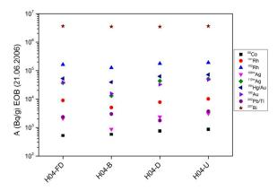
**Fig. 1:** Distribution of radionuclides, which were found in the bulk LBE, taken from segment H04.
