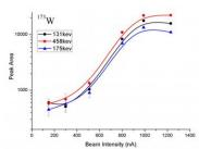
**Fig. 2:** Yield of <sup>173</sup>W, formed in the <sup>19</sup>F + <sup>nat</sup>Tb reaction as a function of beam intensity.
