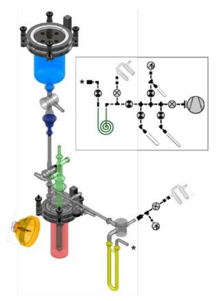
**Fig. 1:** The extraction setup: melting vessel (blue), filtration unit (dark blue), photo-reactor (red), UV lamp (orange), degassing and cooling finger (green) and water trap (yellow). The inset shows the vacuum line for cryogenic trapping and sampling the CO<sub>2</sub> from the photo-reactor, it is connected to the setup at the asterisk (dark green: CO<sub>2</sub> trap).
