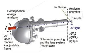
**Fig. 1:** Schematic presentation of the UV-laser module ( $\lambda = 375$  nm) attached on the viewport of the hemispherical electron energy analyzer and aligned on the sample through the electrostatic lens system.
