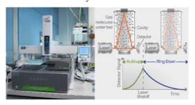
Fig. 1: (Left) L2130-i Picarro laser spectrometer, consisting of an autosampler, vaporizer of the liquid samples, cavity, wash stations to clean the syringe (milli-Q water and methylpyrrolidinone solution), two pumps for the sample removal, hardware and analyzer software. To keep a continuous flow,  $N_2$  is flushed into the system during the measurement cycle. (Right) Scheme of the WS-CRDS technique.
