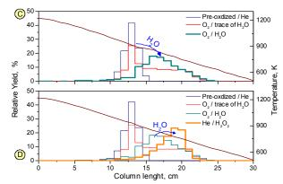
**Fig. 2:** (C) TCm of TeO<sub>2</sub> using O<sub>2</sub>/H<sub>2</sub>O as carrier gas (green bars); (D) TCm of a TeO<sub>2</sub> using as carrier gas He/H<sub>2</sub>O<sub>2</sub> (orange bars).
