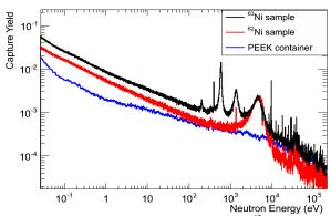
**Fig. 1:** Neutron capture yield of the <sup>63</sup>Ni sample (black) compared to the empty sample container (blue) and a <sup>62</sup>Ni sample (scaled to the <sup>62</sup>Ni content in the <sup>63</sup>Ni sample) [4].
