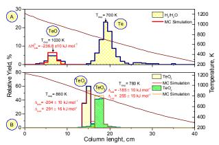
**Fig. 1:** (A) TCm of Te and TeO using as carrier gas  $H_2/H_2O$ ; (B) TCm of  $TeO_2$  and  $TeO_3$  using as carrier gas dry  $O_2$ .
