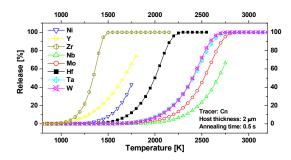
Fig. 2: Calculated release yield of Cn out of 2  $\mu$ m thick catching material at 0.5 s annealing time versus the annealing temperature.
