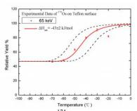
Fig. 4: Yield curve for <sup>174</sup>Os in an isothermal Teflon column
