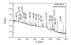
Fig. 2: γ-spectrum of a steel sample (H05-D6-b)
