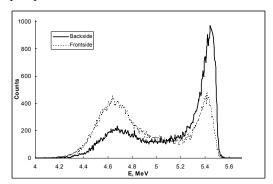
Fig. 1: Alpha-particle spectrum of <sup>241</sup>Am/Rh target.
