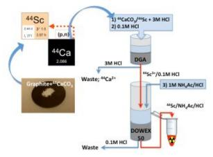
**Fig. 1**: <sup>44</sup>CaCO<sub>3</sub>/graphite target and scheme of the separation procedure of the irradiated target.
