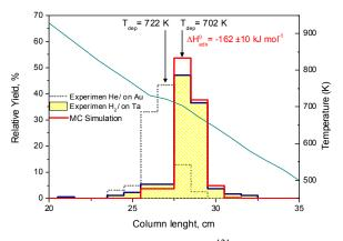
**Fig. 1:** Thermochromatogram of  $^{121m}$ Te deposited on gold using as He (grey dots) and on tantalum using as carrier gas H<sub>2</sub> (yellow bars). The solid red line represents the Monte Carlo simulation of the Te deposited on tantalum.
