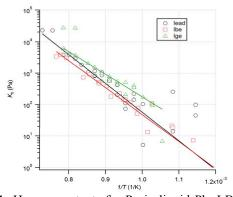
**Fig. 1:** Henry constants for Po in liquid Pb, LBE and LGE. Symbols: data, Solid lines: relations derived from fitting the experimental release curves.
