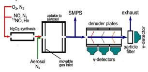
Fig. 1: The new experimental setup: separate  $N_2O_5$  and aerosol reactors are used to allow for improved  $N_2O_5$  production.
