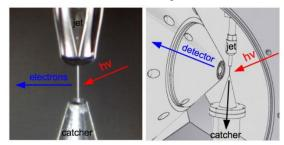
**Fig. 1:** Left: Photograph of the liquid-microjet in action; right: detail of the measurement configuration.
