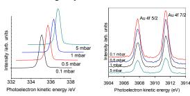
**Fig. 2:** Left: Normalised N1s spectra taken at 735 eV photon energy (SIM) at different gas phase N<sub>2</sub> pressures. The spectra are offset in x- and y-direction for clarity. Right: Au 4f spectra of a gold foil taken at 4000 eV (PHOENIX) at different N<sub>2</sub> pressures. The spectra are background subtracted and offset in y-direction for clarity.
