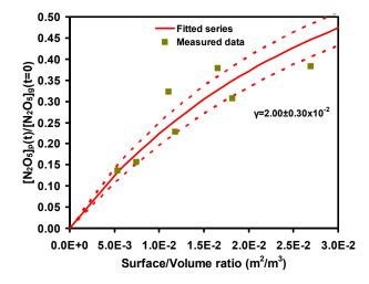
**Fig. 2:** Data set collected using citric acid aerosol at 61.5% RH. Green squares represent measured data points while the red curve is a fit to the data according to the kinetic model, with the dotted curve showing the error range
