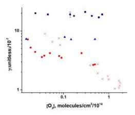
**Fig. 2:** Uptake coefficient  $\gamma$  vs.  $[O_3]$  for mixed NaBr/CA films with bromide concentrations of 4M (squares), 0.34M (triangles) and 84mM (circles), respectively, at 72% RH and 20°C. Red crosses denote data from Oldridge and Abbatt [2] (8.6mM bromide in NaCl solution).
