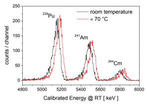
**Fig. 2:** α-spectra of a three-line source at room temperature and with a resistively heated Ta wire in 10 cm distance ( $T_{wire} > 1000$ °C,  $T_{det} \approx 70$ °C); the energy resolution remained at  $\approx 80$  keV (FWHM).
