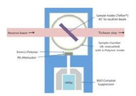
Fig. 1: Schematic view of the used PGAA setup
