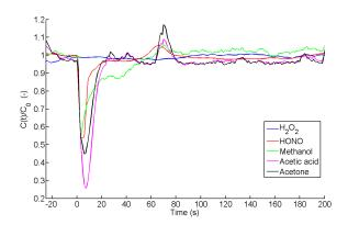
**Fig. 2:** Relative gas-phase concentration of various trace gases with time upon exposure to fluorinated ethylene propylene (FEP). At t=0s low concentrations of the sample gas were exposed to fluorinated polymers at 223 K to 253 K.
