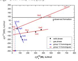
Fig. 1: Stability trends for group 12 and 14 sulfides.
