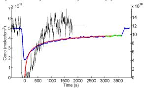
**Fig. 1:** Gas phase concentration of  $H_2O_2$  (blue line, left axis) and  $HNO_4$  (black line, right axis) with time. Between t=0 s and 3560 s the  $H_2O_2$  is passed over the ice. Also shown is an asymptotic fit (red line) to the later part of the uptake data (green line) for  $H_2O_2$ .
