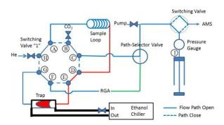
**Fig. 1:** Instrumental setup. Red color indicates CO<sub>2</sub> during loading and elution. Green line or RGA were disconnected during breakthrough or release experiments respectively.
