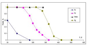
**Fig. 2:** Decomposition curves for <sup>104</sup>Mo carbonyl on different surfaces.
