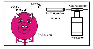
Fig. 1: Experimental setup for carbonyl decomposition studies.
