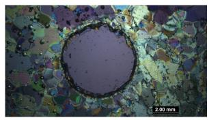
**Fig. 2:** A flow tube (blue-grey circle) drilled in to a polycrystalline ice block.
