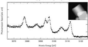
**Fig. 2:** Ce 3d XPS spectrum in an O<sub>2</sub> atmosphere (1.0 mbar, 298 K), taken at 6 keV photon energy. Inset: TEM image of the catalyst (2wt%Pt/CeO<sub>2</sub>). The image width is 50 nm.
