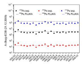
**Fig. 2:** Measured activity concentrations of <sup>208-210</sup>Po in Bq/g at EOB (21.12.2006) for different MEGAPIE samples compared to FLUKA predictions.
