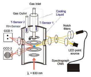
Fig. 1: Electrodynamic balance
