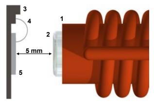
**Fig. 1:** Test setup for isothermal vacuum chromatography with carrier-free <sup>211</sup>Pb; **1** isothermal oven, **2** quartz column exit, **3** ceramic carrier, **4** wire bonds. **5** CVD diamond detector.
