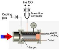
**Fig. 1:** Set-up used for the synthesis and transport of carbonyls at the IMP cyclotron.
