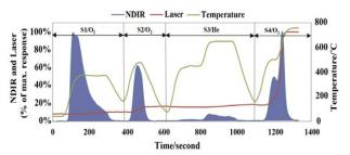
Fig. 1: A typical thermogram of a water-extracted aerosol sample (Solothurn) by the Swiss 4S protocol.
