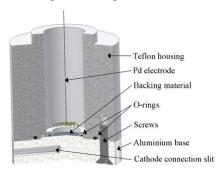
Fig. 1: Electrodeposition cell.
