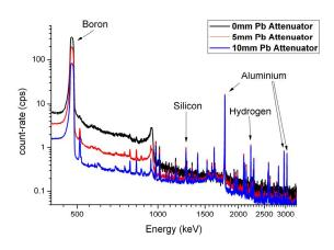
Fig. 2: Low-energy part of the measured PGAA spectra
