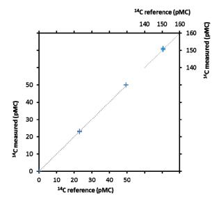
**Fig. 2:** Double <sup>14</sup>C analysis of the reference materials IAEA C4, C5, C6 and C7. Measurement uncertainties range from 0.2 to 0.5 pMC.
