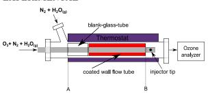
Fig. 1: A schematic diagram of the flow tube system used in  $O_3$  uptake measurements to the coated film.
