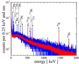
**Fig. 1:** γ-spectrum of a sediment sample (blue line; total mass 4.5 g, 72 h measurement period) and background spectrum (red line, 1000 h measurement period) recorded with active anti-cosmic shield.
