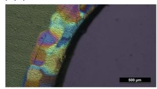
**Fig. 3:** The edge of a flow tube (blue-grey) drilled into a single crystalline ice block (greenish).
