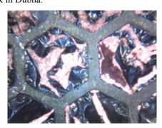
**Fig. 2:** Optical microscopy image of the <sup>243</sup>Am/Ti target after irradiation.
