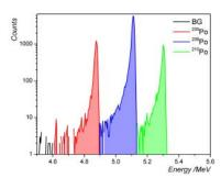
**Fig. 1:** Typical spectrum of deposited <sup>208/209/210</sup>Po - peak areas for integration are colored.
