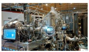
**Fig. 1:** The NAPP endstation hooked up at the SIM beamline at SLS, with the liquid jet chamber attached.
