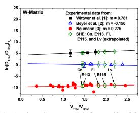
**Fig. 1:** The volume approach from Bakker [5] as  $\ln(D_{Trac}/D_{Self})$  versus  $V_{Trac}/V_{Host}$  given for tungsten as host material at its melting temperature ( $\theta=1.00$ ). The plot includes literature data [1,2,3]. The hollow rectangles with the error bars ( $1\sigma$ ) are calculated values for the SHE with  $112 \le Z \le 116$ . m: slope of the linear regressions.
