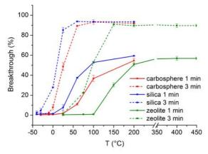
**Fig. 2:** Breakthrough of  $CO_2$  (45  $\mu$ gC) from the traps.
