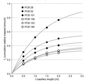
**Fig. 1:** Cumulated relative trapped amounts  $-f_c$  (points) and fraction of total amount  $-f_{tot}$  (grey lines) of  $^{13}C_{12}$ -labeled PCB congeners in the capillary segments relative to the set concentrations in the water sample [3].
