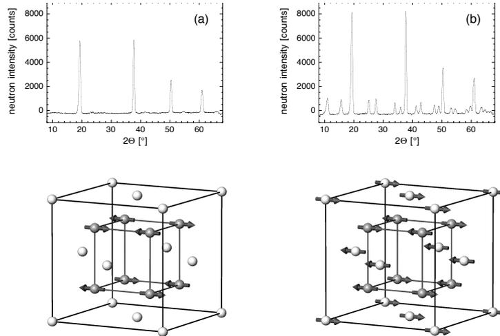
Figure 4: (a) Neutron diffraction pattern (magnetic scattering only) and corresponding magnetic structure in  $\text{Nd}_3\text{Pd}_{20}\text{Ge}_6$  below  $T_{N1} = 1.75$  K. While the Nd moments on one site are antiferromagnetically ordered, the moments on the other site remain disordered. (b) Magnetic neutron diffraction pattern and corresponding magnetic structure below  $T_{N2} = 0.58$  K; also the second Nd sublattice is magnetically ordered.
