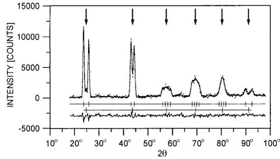
Figure 6: ErGa<sub>3</sub>: Observed (points) and calculated (line) magnetic difference neutron diffraction pattern showing the magnetic peaks only (satellites). The arrows indicate the nuclear peak positions.
