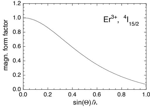
Figure 2: Magnetic form factor for the trivalent rare-earth ion Er<sup>3+</sup> (dipole approximation) with ground state <sup>4</sup>I<sub>15/2</sub>.
