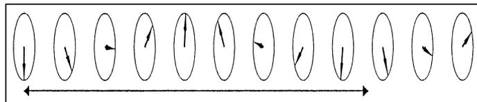
Figure 5: Schematic view of a simple spiral magnetic structure (helix). The long horizontal arrow shows the repeat distance.
