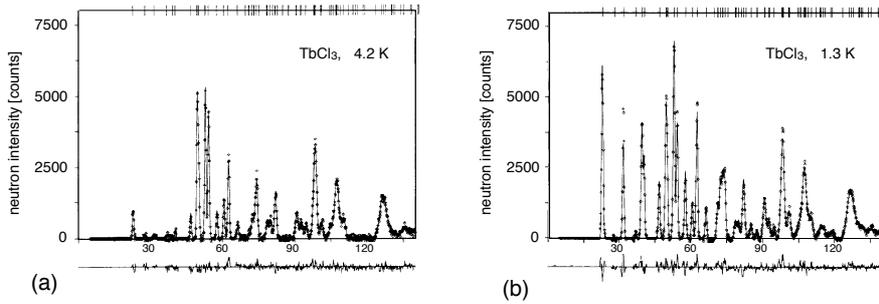
Figure 3: (a) Observed (points, a linear background has been subtracted) and calculated (line) neutron diffraction intensities of paramagnetic  $\text{TbCl}_3$  at 4.2 K. (b) Observed (points) and calculated (line) neutron diffraction patterns of ferromagnetic  $\text{TbCl}_3$  at 1.3 K.
