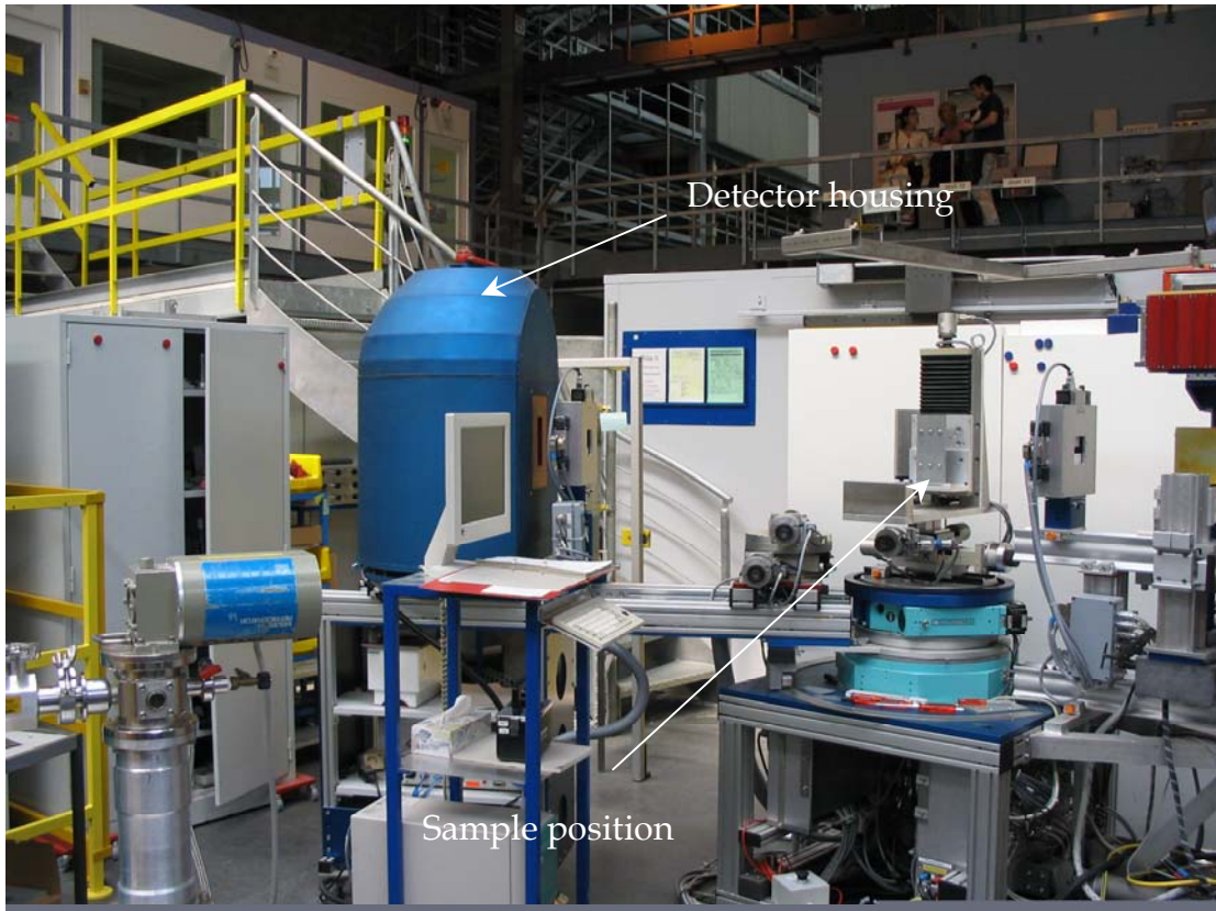
Figure 12. Side view of MORPHEUS experimental setup
