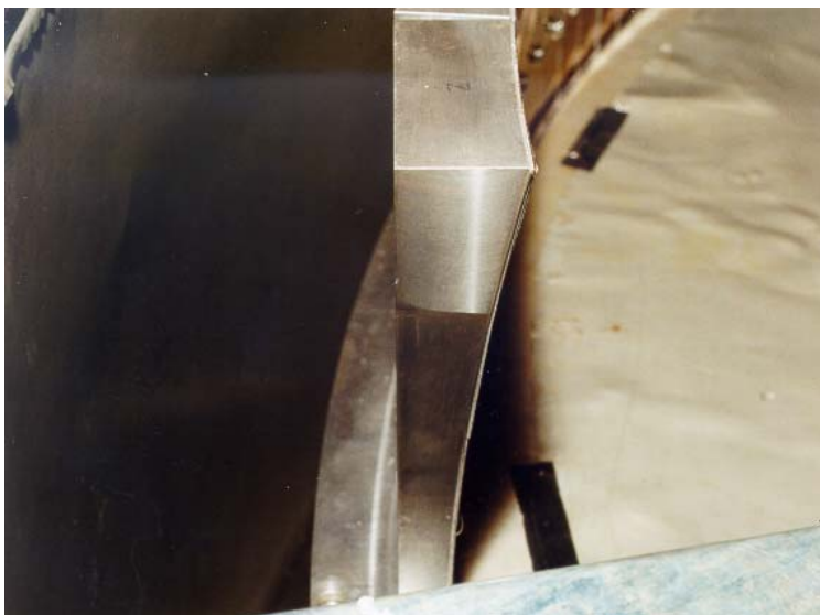
Figure. 5 The curved profile of the mica backing plates
