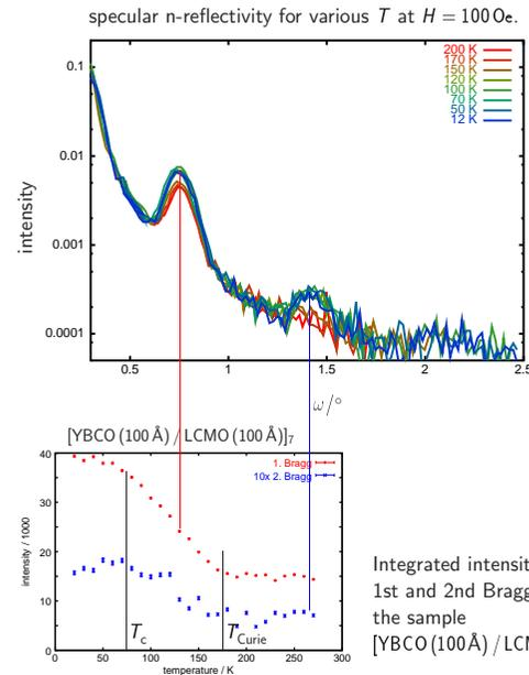
Integrated intensities of the 1st and 2nd Bragg peak of the sample  $[\text{YBCO}(100\text{ \AA}) / \text{LCMO}(100\text{ \AA})]_7$
