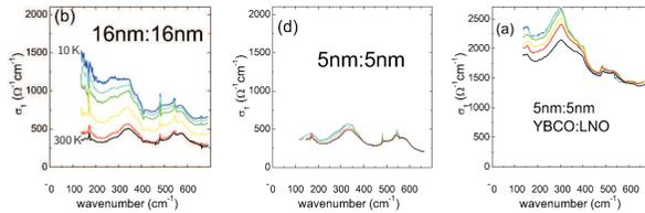
Representative spectra for the real-parts of the in-plane conductivity  $\sigma_1$  of YBCO/LCMO multilayers obtained by ellipsometry [1].
