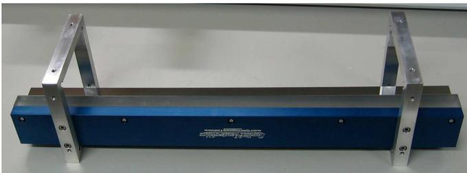
Figure 7: Single guide element (half a guide section). The blue part is an L-shaped Al bar on which the glass substrates are screwed. The Al frames are for mounting the elements on the support and alignment system.
