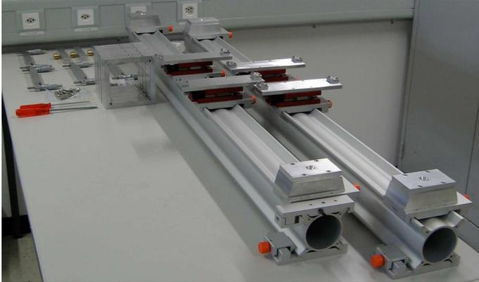
Figure 5: Parts of the guide support before mounting the guide elements.
