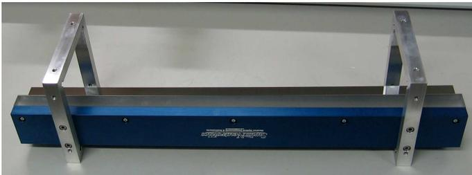
Figure 20: Single guide element (half a guide section). The blue part is an L-shaped Al bar on which the glass substrates are screwed. The Al frames are for mounting the elements on the support and alignment system.
