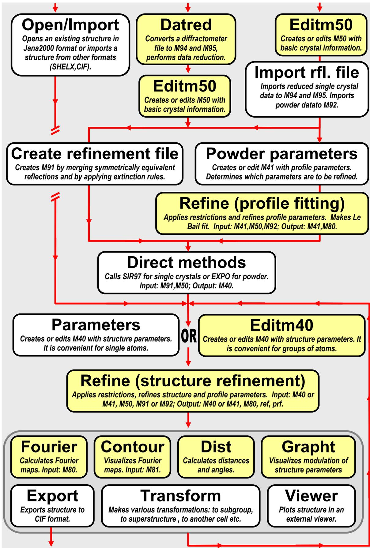
The yellow boxes indicate tools that are started through an icon in the basic window of Jana2000. The tools shown in the white boxes are started through a menu. Only the most important input and output files are shown.
