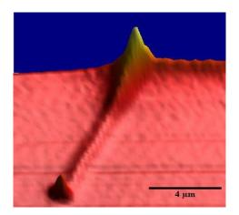
Spatial carrier diffusion and optical waveguiding in a ZnO nanowire in response to point source e beam excitation.
