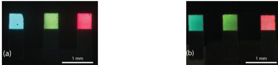
Figure 7: Tri-color pixels imaged using a light microscope are shown for an Al / TBA cathode at 20 V (a) and for an Al cathode at 24 V (b).
