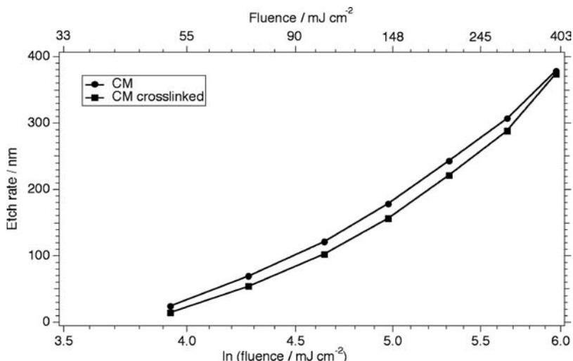
**Fig. 81** Ablation rates per pulse,  $d$ , as a function of the laser fluence,  $F$ , for the CM and  $CM_{\text{cross}}$  polymer. REPRINTED WITH PERMISSION OF [Ref. 120], COPYRIGHT (2000) Wiley-VCH Verlag GmbH
