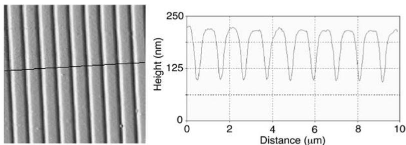
**Fig. 89** AFM image of grating of 1090-nm spacing. 1 pulse with  $80 \text{ mJ cm}^{-2}$  with the X-Z plot as *insert*. REPRINTED WITH PERMISSION OF [Ref. 326], COPYRIGHT (1999) American Institute of Physics
