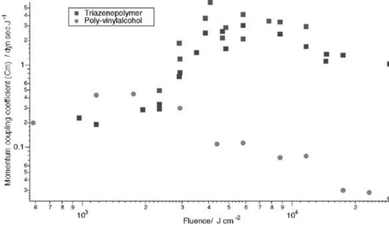
**Fig. 100** Momentum coupling coefficients (impulse/laser energy) at various fluences for the carbon-doped polymers. Optical density at 935 nm  $\approx 0.9$ , film thickness  $\approx 65 \mu\text{m}$ , PET substrates. REPRINTED WITH PERMISSION OF [Ref. 222], COPYRIGHT (2001) Elsevier Science
