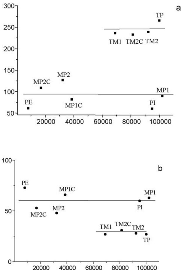
**Fig. 9** Influence of the linear absorption coefficients at the laser wavelength on **a** the etch rates at  $100 \text{ mJ cm}^{-2}$  and on **b** the threshold fluences. The *lines* in the figure are just for guiding the eyes. REPRINTED WITH PERMISSION OF [Ref. 82], COPYRIGHT (2001) American Chemical Society
