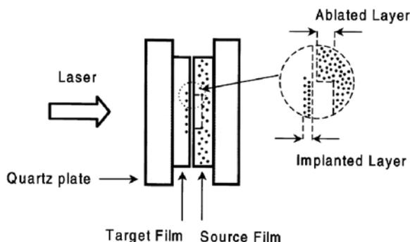
**Fig. 83** Schematic diagram of the laser-induced molecular transfer process. REPRINTED WITH PERMISSION OF [Ref. 360], COPYRIGHT (1998) Elsevier Science
