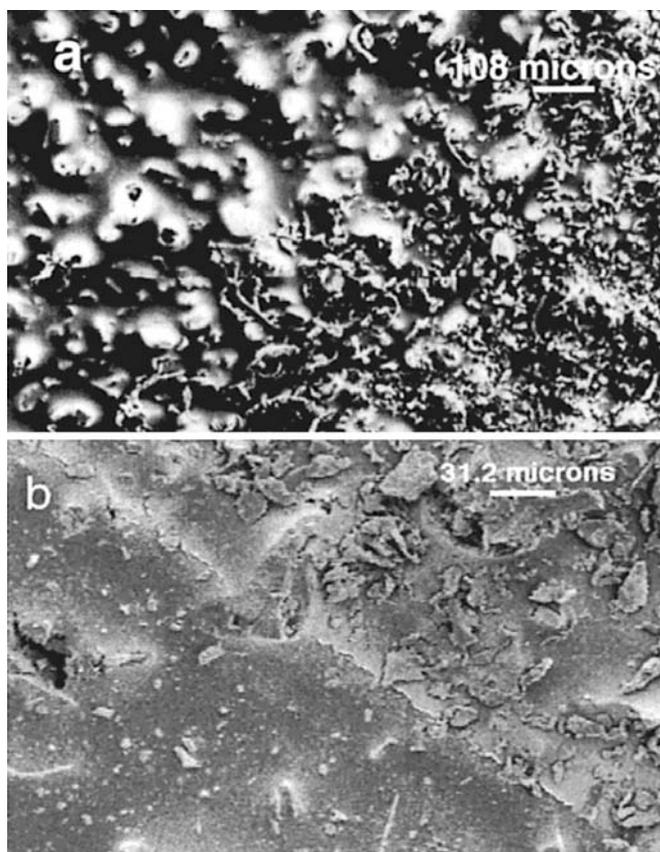
**Fig. 60** Scanning electron microscopy (SEM) pictures of a SiC disk. **a** In the *lower right* part of the picture the abraded Kapton is visible as scrapes. **b** The border between laser-treated and untreated area is shown. The *lower left* side corresponds to the laser-treated area (20 pulses at  $155 \text{ mJ cm}^{-2}$ ). REPRINTED WITH PERMISSION OF [Ref. 135], COPYRIGHT (2000) American Chemical Society
