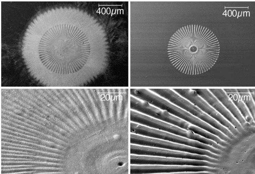
**Fig. 94** SEM images of Siemens stars fabricated by laser ablation. *Top*: Siemens stars in polyimide (*left*) and in the triazene polymer (*right*) using 5 pulses. *Bottom*: magnification of the Siemens stars in the top row. REPRINTED WITH PERMISSION OF [Ref. 322], COPYRIGHT (2001) Elsevier Science
