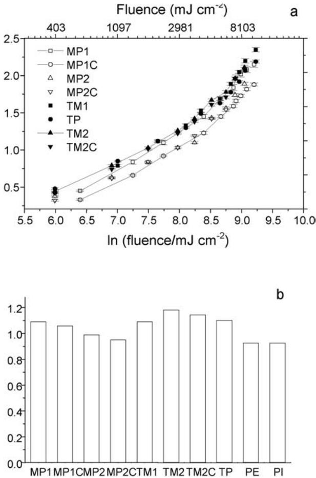
**Fig. 3. a** Measured etch rates as a function of natural logarithm fluence at high fluences (0.5 to 10  $\text{J cm}^{-2}$ ). **b** Calculated etch rates of all polymers at 2,000  $\text{mJ cm}^{-2}$ . REPRINTED WITH PERMISSION OF [Ref. 82], COPYRIGHT (2001) American Chemical Society
