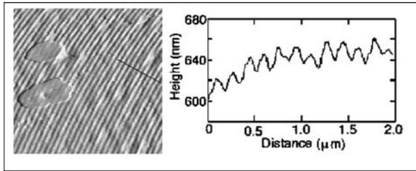
**Fig. 90** AFM image of grating of 180-nm spacing, 1 pulse with  $155 \text{ mJ cm}^{-2}$  with the X-Z plot as *insert*. The curvature of the grating lines is an experimental artifact. REPRINTED WITH PERMISSION OF [Ref. 326], COPYRIGHT (1999) American Institute of Physics
