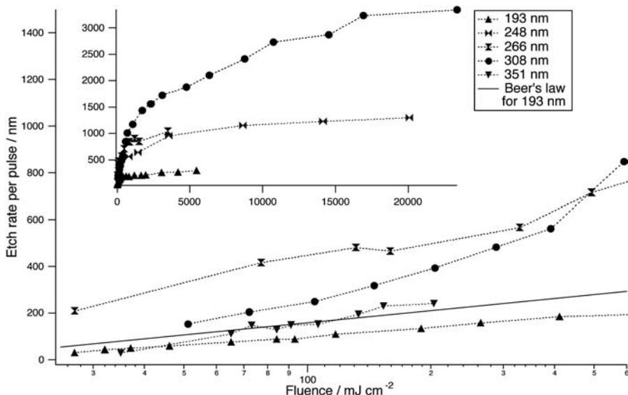
**Fig. 73** Measured etch rates of TP vs the logarithm of the fluence (up to  $600 \text{ mJ cm}^{-2}$ ) for different irradiation wavelengths. *Insert* shows the same plot for the complete linear fluence range. REPRINTED WITH PERMISSION OF [Ref. 221], COPYRIGHT (2002) Elsevier Science
