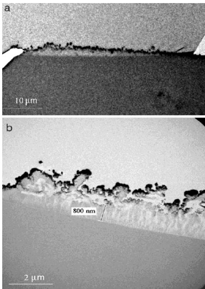
**Fig. 75** TEM micrographs of the transverse section of the line structure obtained with 800 pulses at  $80 \text{ mJ cm}^{-2}$ , showing the edge of the crater (at the *far left* of the micrographs). **a** Overall view of the profile of the deposited material. The width of the region is  $36 \mu\text{m}$ . **b** The section near the edge of the crater, showing the details of the deposited material. REPRINTED WITH PERMISSION OF [Ref. 132], COPYRIGHT (2000) American Institute of Physics
