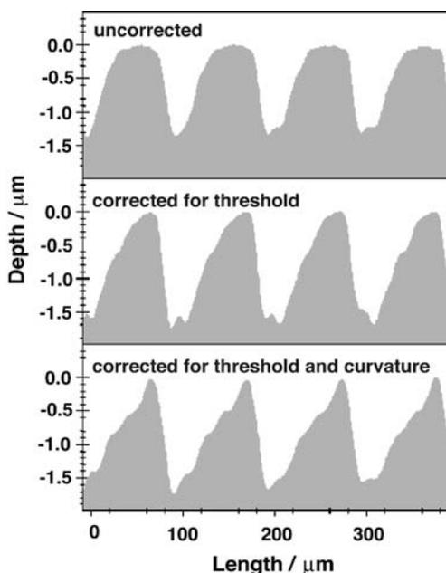
**Fig. 93** Profilometer scans of blazed grating structures ablated into polyimide. The profile shape depends on the corrections for the polymer response, i.e., etch rate per pulse at a given fluence. REPRINTED WITH PERMISSION OF [Ref. 322], COPYRIGHT (2001) Elsevier Science
