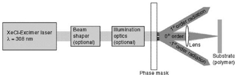
**Fig. 92** Setup for the patterning of polymer surfaces by laser ablation using diffractive masks. REPRINTED WITH PERMISSION OF [Ref. 322], COPYRIGHT (2001) Elsevier Science
