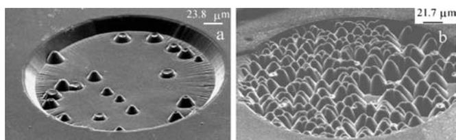
**Fig. 6** SEM micrographs of ablated craters at low fluences. **a** Crater in TM2, irradiated at  $69 \text{ mJ cm}^{-2}$  with 88 pulses. **b** Crater in MP2C irradiated at  $51 \text{ mJ cm}^{-2}$  with 200 pulses. REPRINTED WITH PERMISSION OF [Ref. 82], COPYRIGHT (2001) American Chemical Society
