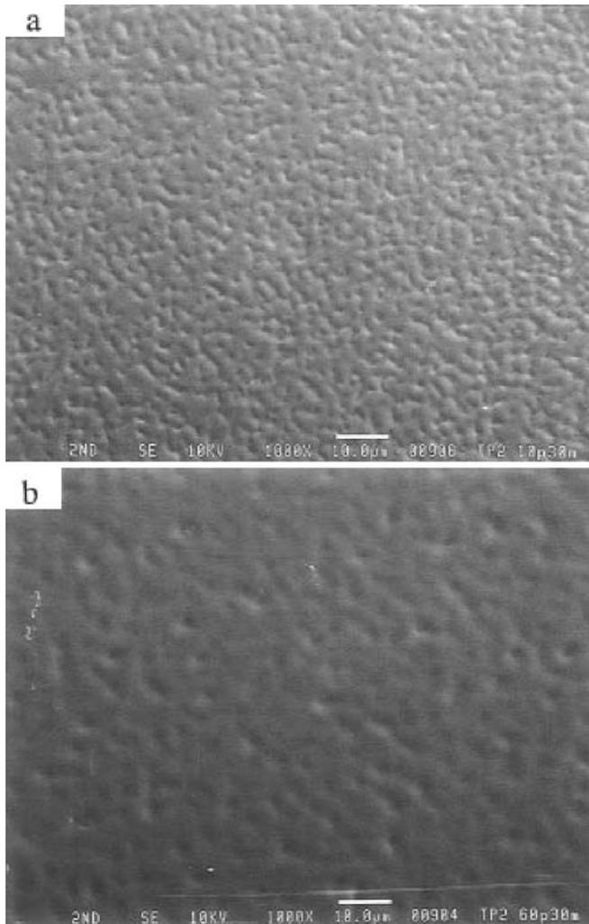
**Fig. 11** Scanning electron micrographs of surface changes. **a** after 10 pulses with  $30 \text{ mJ cm}^{-2}$  at 308 nm and **b** after 60 pulses with  $30 \text{ mJ cm}^{-2}$  at 308 nm. REPRINTED WITH PERMISSION OF [Ref. 62], COPYRIGHT (1996) American Chemical Society
