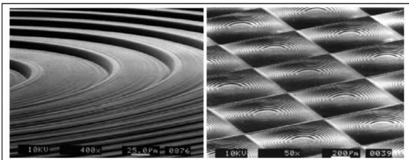
**Fig. 95** SEM micrograph of diffractive lens structures ablated into polyimide (*left*, lens diameter 2.5 mm) and array of lens structures (using a step and repeat mode, lens dimensions  $900 \times 900 \mu\text{m}$ ). REPRINTED WITH PERMISSION OF [Ref. 322], COPYRIGHT (2001) Elsevier Science
