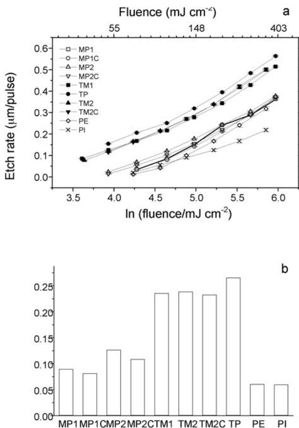
**Fig. 5. a** Etch rates at low fluences (up to  $400 \text{ mJ cm}^{-2}$ ) as a function of the natural logarithm of the laser fluence. **b** Calculated etch rates at  $100 \text{ mJ cm}^{-2}$  for all polymers. REPRINTED WITH PERMISSION OF [Ref. 82], COPYRIGHT (2001) American Chemical Society
