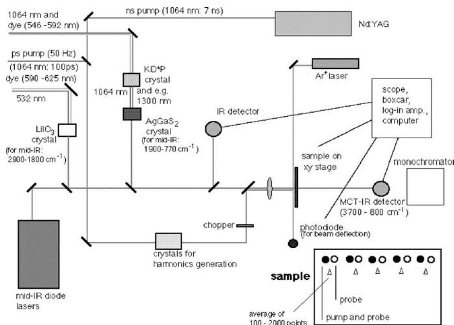
**Fig. 54** Detailed scheme of the setup in the sample area
