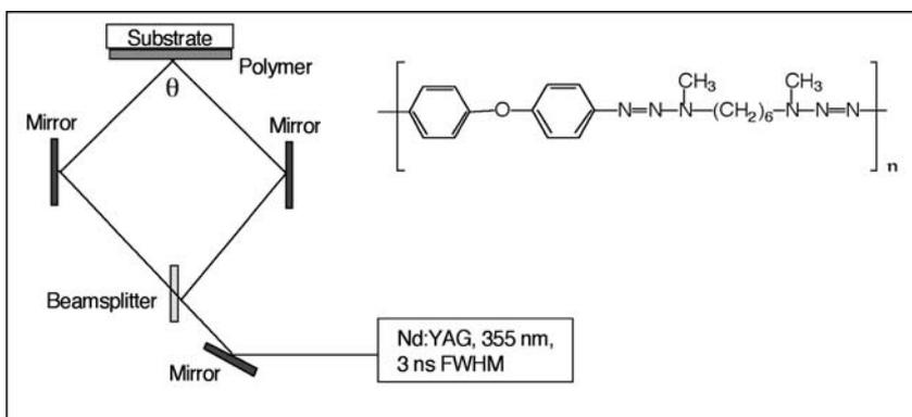
**Fig. 88** Experimental setup with inserts of the chemical structure of the polymer. REPRINTED WITH PERMISSION OF [Ref. 326], COPYRIGHT (1999) American Institute of Physics
