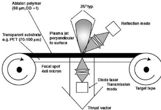
**Fig. 99** Scheme of the possible design for LPTs. REPRINTED WITH PERMISSION OF [Ref. 222], COPYRIGHT (2001) Elsevier Science
