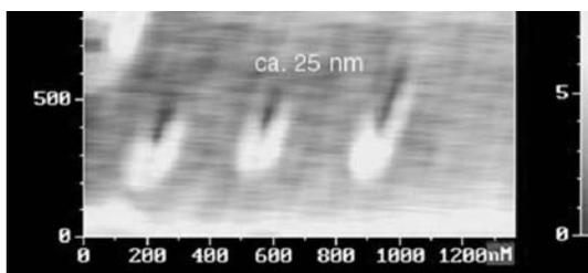
**Fig. 97** Nanostructures in the laser-softened triazene polymer. The structuring was performed by moving the AFM tip from the upper part downwards. The image was taken in the noncontact mode of the same AFM instrument
