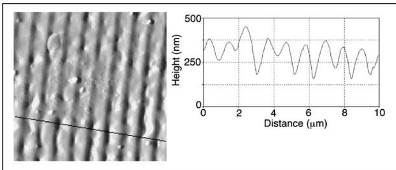
**Fig. 91** AFM image of grating of 1090-nm spacing, 5 pulses with  $80 \text{ mJ cm}^{-2}$  with the X-Z plot as *insert*. REPRINTED WITH PERMISSION OF [Ref. 326], COPYRIGHT (1999) American Institute of Physics
