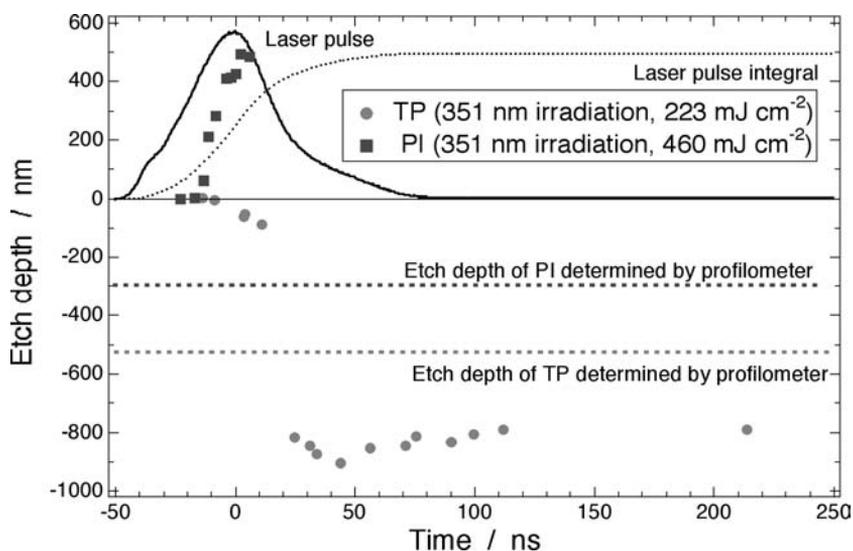
**Fig. 76** Nanosecond expansion/etching behavior of the triazene polymer and polyimide after 351-nm irradiation. REPRINTED WITH PERMISSION OF [Ref. 221], COPYRIGHT (2002) Elsevier Science
