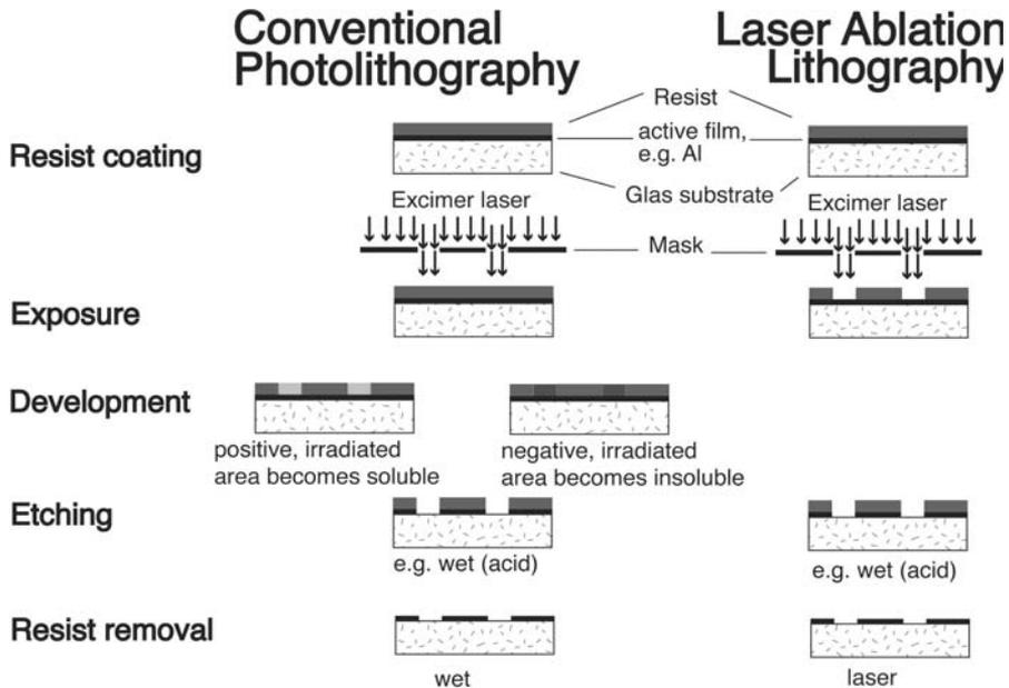
**Fig. 2** Comparison between the process steps for conventional lithography and laser ablation lithography
