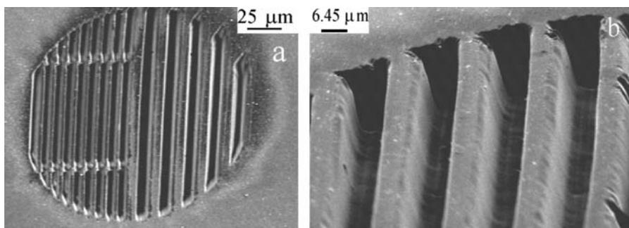
**Fig. 7** SEM micrographs of microstructures. **a** Structure in MP2C irradiated at  $4.6 \text{ J cm}^{-2}$  with 9 pulses. **b** Structure in TM2C irradiated at  $4.6 \text{ J cm}^{-2}$  with 11 pulses. REPRINTED WITH PERMISSION OF [Ref. 82], COPYRIGHT (2001) American Chemical Society
