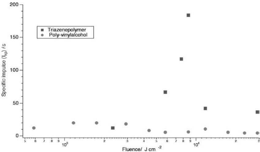
**Fig 101** Specific impulse at various fluences for the carbon-doped polymers. Same materials as in Fig. 100. REPRINTED WITH PERMISSION OF [Ref. 222], COPYRIGHT (2001) Elsevier Science
