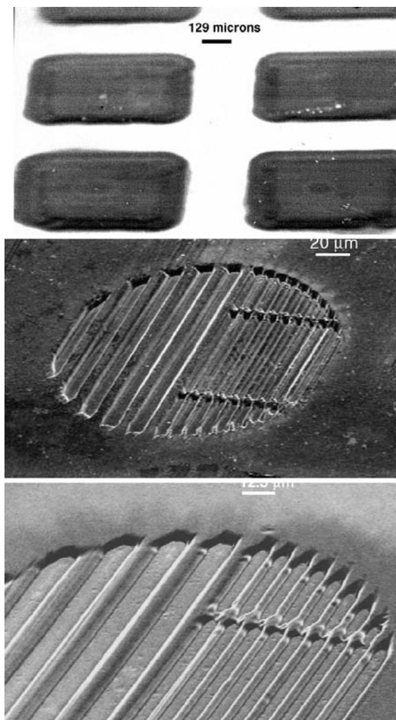
**Fig. 82** SEM pictures of the CM polymer after cross-linking. *Top*: after wet development in  $\text{CHCl}_3$ ; *middle*: structuring of the cross-linked and wet developed polymer (from top SEM) (1 pulse with  $7.9 \text{ J cm}^{-2}$  at 308 nm); *bottom*: inverse processing, i.e., first laser structuring, then cross-linking and wet development. REPRINTED WITH PERMISSION OF [Ref. 120], COPYRIGHT (2000) Wiley-VCH Verlag GmbH
