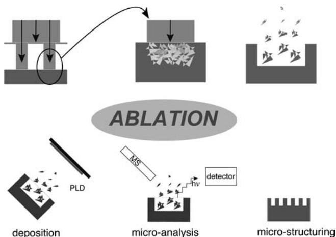
**Fig. 1** Different applications of laser ablation
