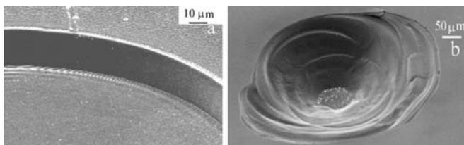
**Fig. 4** SEM micrographs of craters ablated with high fluences. **a** TM2 irradiated at  $8.5 \text{ J cm}^{-2}$  with 10 pulses. **b** MP2C irradiated at  $7.3 \text{ J cm}^{-2}$  with 11 pulses. REPRINTED WITH PERMISSION OF [Ref. 82], COPYRIGHT (2001) American Chemical Society
