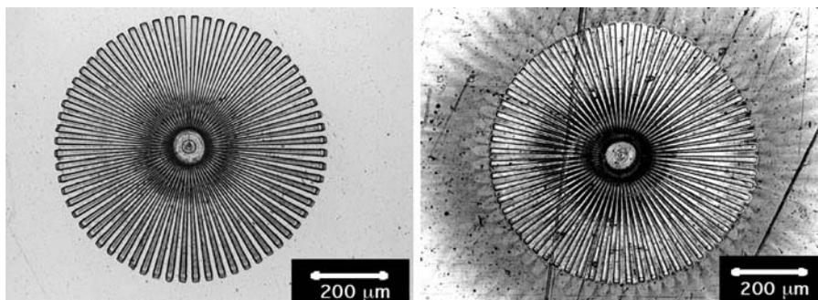
**Fig. 74** SEM images of Siemens stars fabricated by laser ablation. Siemens stars in the triazene polymer (*left*) and in polyimide (*right*) using 5 pulses. REPRINTED WITH PERMISSION OF [Ref. 221], COPYRIGHT (2002) Elsevier Science
