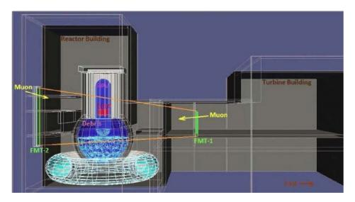
**Figure 1.20.:** *Schematics of one Fukushima reactor with muon detectors.*
