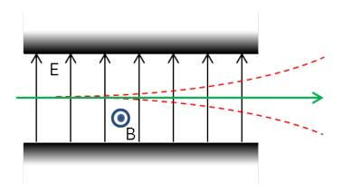
**Figure 1.42.:** Schematic of a Wien filter. The particles following the green trajectory will have the chosen velocity. The one with a lower (higher) velocity will be deflected on the top (bottom) of the figure.
