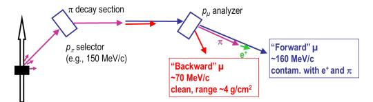
**Figure 1.33.:** Principle of a high energy beamline (as  $\mu E1$  at PSI). In practice "backward" muon beams are used which are less energetics but are much less contaminated by other particles. For high-pressure experiments, one usually use momentum up to 110 MeV/c.
