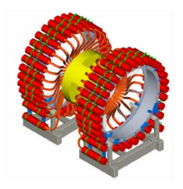
**Figure 3.10.:** Schematic view of a  $\mu$ SR instrument at a pulsed beam. The red cylinders are photomultipliers connected to positron detectors (here 64 in total, "MUSR" instrument at ISIS). The diameter of the frame where the photomultipliers are mounted is more than one meter. Newer instruments can have up to 600 detectors.
