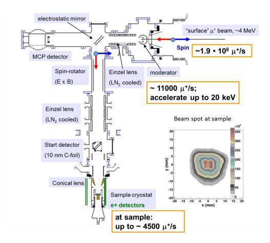
**Figure 7.7.:** Low energy polarized muon beam generated via moderation and  $\mu$ SR spectrometer for experiments on thin films, multilayers and near surface regions at the Paul Scherrer Institute.
