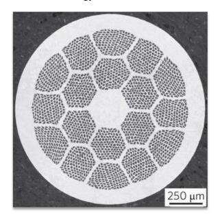
**Figure 6.6.:** Cross-section of a superconducting wire made of Bi-2212 material (high- $T_c$  material). The superconducting filaments are the small black dots, which are embedded in a copper matrix (see Ref [72] for details).
