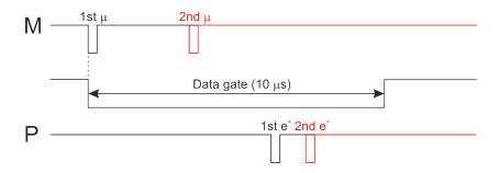
**Figure 3.8.:** Timing diagram of a  $\mu$ SR measurement at a cw beam. Here we assume that all the muon events have passed the logic condition defined above. The first muon will start the clock and the data gate. In this data gate only one positron has to be detected. If a 2nd muon or a 2nd positron is detected then the full set of events is rejected. Note that the 1st muon is actually a "good muon" only if there was no other muon event in the past for at least the length of the data gate.
