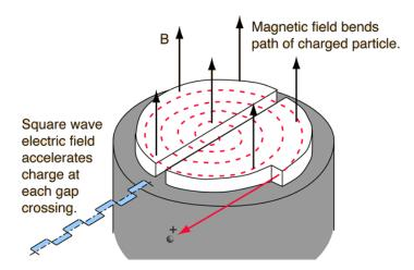
**Figure 1.23.:** *Cyclotron: operation principle.* (*Taken from* http://hyperphysics.phy-astr.gsu.edu/hbase/magnetic/cyclot.html).
