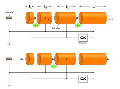
**Figure 1.22.:** *Schema of a linear accelerator.* (*Taken from* https://en.wikipedia.org/wiki/Linear\_particle\_accelerator).
