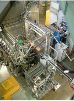
**Figure 7.10.:**  $\mu$ SR LEM instrument in the  $\mu$ E4 area at PSI. Left: last section of the high intensity surface muon beam feeding the LEM apparatus. Right: LEM Apparatus. The surface muons are coming from the right. The moderator cryostat with the 90° deflection as well as the  $\mu$ SR spectrometer and sample chamber in the lower part of the picture are visible.
