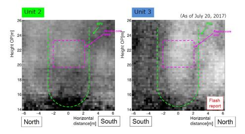
**Figure 1.21.:** Comparisons between measurements performed for the Reactors 2 and 3. Whereas indications are present that fuel is located in the Reactor Pressure Vessel (RPV) for the unit 2, no indication of spent fuel is so far observed for the unit 3.
