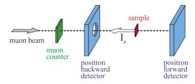
**Figure 3.11.:** Zero-field (ZF)  $\mu$ SR geometry. In reality, the detectors are located about 2 cm away from the sample. The denomination of the detectors refers to the beam direction. Adapted from P. Dalmas de Réotier and A. Yaouanc [31].
