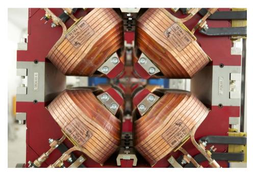
Figure 1.38.: Typical quadrupole magnet.
