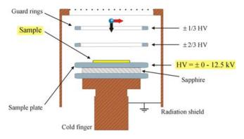
**Figure 7.9.:** Low energy polarized muon beam generated via moderation and  $\mu$ SR spectrometer for experiments on thin films, multilayers and near surface regions at the Paul Scherrer Institute.
