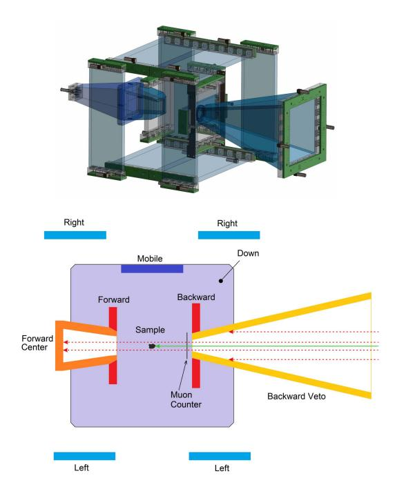
**Figure 3.7.:** Schematic view of a typical  $\mu$ SR detector setup at a continuous beamline (Instrument GPS at PSI [30]). Top: 3D-view of the muon and positron detectors where the SiPM-readout is visible. Bottom: Cross-section at the sample level (top view). The muons are entering the spectrometer from the right-hand side, i.e. parallel to the axis of the Backward veto pyramid. The lateral dimension of the Down detector is 10 cm.
