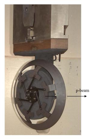
**Figure 1.27.:** *Photograph of the PSI E graphite target.*
