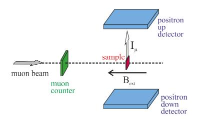
**Figure 3.15.:** Transverse-field (TF)  $\mu$ SR geometry. The externally applied magnetic field is along the muon beam (surface beam) to avoid a beam bending through the Lorentz force. The initial muon spin direction is (ideally) 90° with respect to the beam direction (rotation by a spin rotator up-stream). <sup>12</sup>Adapted from P. Dalmas de Réotier and A. Yaouanc [31].
