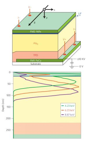
**Figure 7.21.:** Top: A schematic diagram showing the structure of our device. The layers FM1 and FM2 and the two ferromagnetic layers. Bottom: Depth profile showing the calculated probability that a positively charged muon with an implantation energy of 4.23, 6.23 or 8.87 keV (green, orange or purple line) comes to rest at a certain depth within the device (so-called stopping or implantation profile). Taken from Ref. [114].
