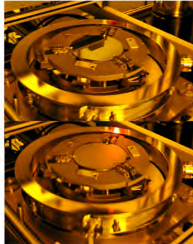
Figure 5.22: Jenoptik HEX03 nanoimprint machine with an integrated adapter for a Süss alignment fixture for an anodic bonder. Alignment is possible by using the appropriate mask aligner.
