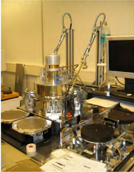
Figure 5.18: Nanoimprint machine from EV Group based on an anodic bonder. Alignment is possible by using an appropriate mask aligner.
