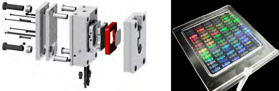
Figure 1: Versatile tooling for rapid variotherm injection molding (left) and sample of security feature replication (right).
