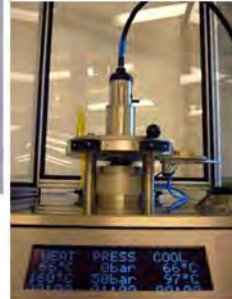
Figure 5.24: Nanoimprint machine from Obducat using a pressurized membrane on one side instead of a hard stamper (call soft imprint – not to be confused with soft lithography). By using a transparent membrane, thermal imprint can be combined with UV-curing.
