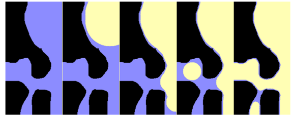
Fig. 2.15: Drainage of an example model structure map for decreasing relative humidity (frames from left to right), considering capillary effects (drainage of core of pores with decreasing radius) and surface adsorption effects (thinning of surface water films). Black: solid, blue: water, yellow: drained pore.
