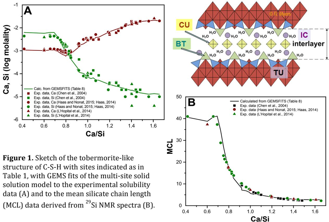
**Figure 1.** Sketch of the tobermorite-like structure of C-S-H with sites indicated as in Table 1, with GEMS fits of the multi-site solid solution model to the experimental solubility data (A) and to the mean silicate chain length (MCL) data derived from  $^{29}\text{Si}$  NMR spectra (B).
