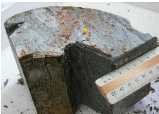
Fig. 4.1: Photograph of ABM Package 1 block 18. The sample was taken in the range from 5 to 15 mm from the boundary of the heater.
