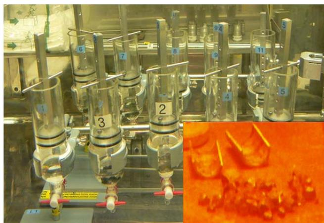
Fig. 2.9: Experimental setup of the spent fuel leaching experiments at PSI. The insert shows spent fuel fragments separated from the cladding.
