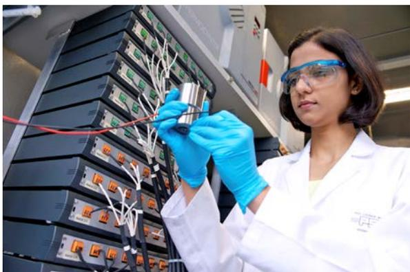
Multi-channel battery testing facilities.
