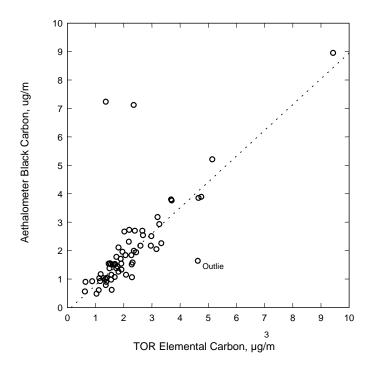
Intercomparison of Aethalometer data with 'TOR' analysis of parallel samples: from Allen, Lawrence, and Koutrakis, "Field Validation...", *Atmos. Env.* **33**: 5 (Feb 1999)
