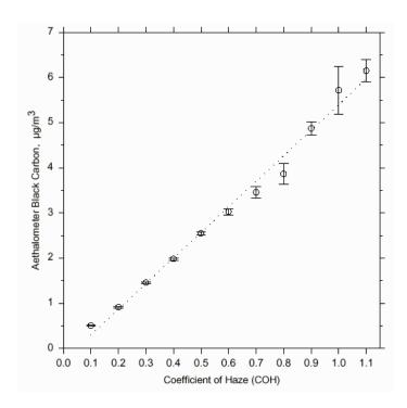
Intercomparison of Aethalometer (µg/m³) with Coefficient Of Haze tape sampler (COH): from Allen, Lawrence, and Koutrakis, "Field Validation...", *Atmos. Env.* **33**: 5 (Feb 1999).
