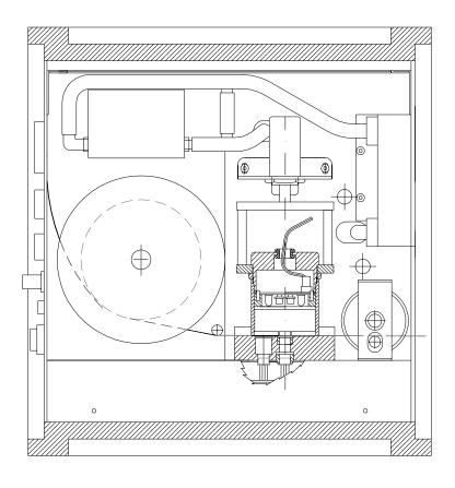
Figure 16: 'Portable' Aethalometer<sup>TM</sup> - left side interior
