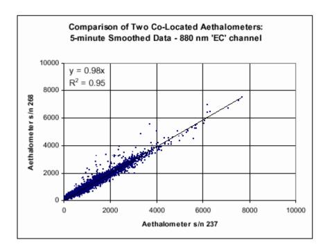
Comparison of data from two co-located Aethalometers under test at the ETV Pittsburgh site.
