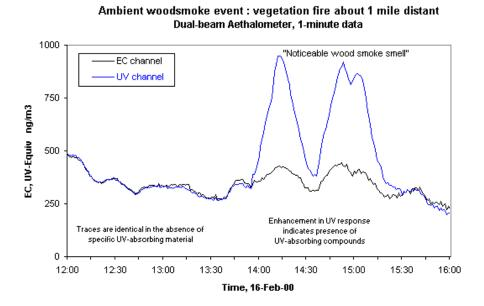
Dual-wavelength Aethalometer data during impact of smoke from burning vegetation.
