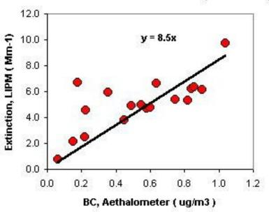
Intercomparison of Aethalometer data (µg/m³) with 'Laser Integrating Plate' analyses (Mm⁻¹)
