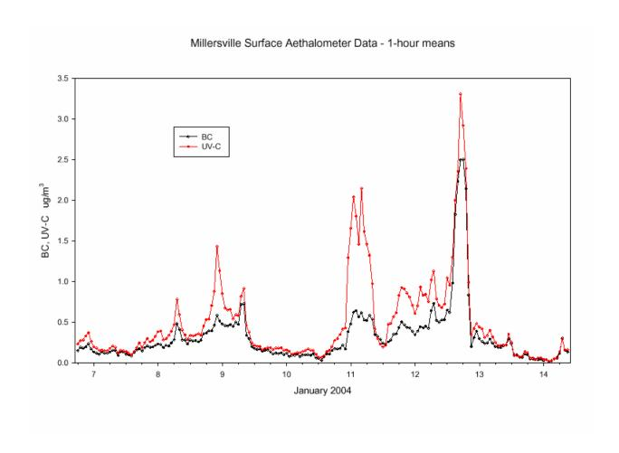
The final figure illustrates 'Spectrum' 7-wavelength Aethalometer data taken in an urban location where the aerosol is essentially uniformly absorbing across the wavelength range from 370 to 950 nm. The tracking of the data in all seven wavelengths vindicates the assumption of the  $1/\lambda$  dependence of absorption.
