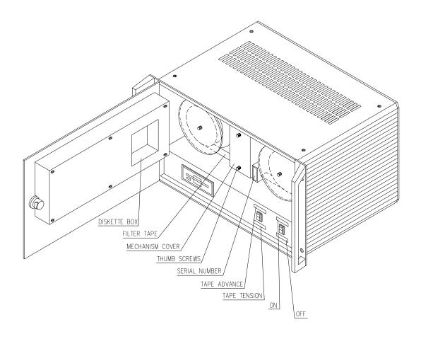
The Aethalometer TM - 19-inch rack mount chassis version
