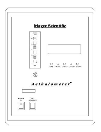
Figure 18: 'Portable' Aethalometer<sup>TM</sup> -fromt view
