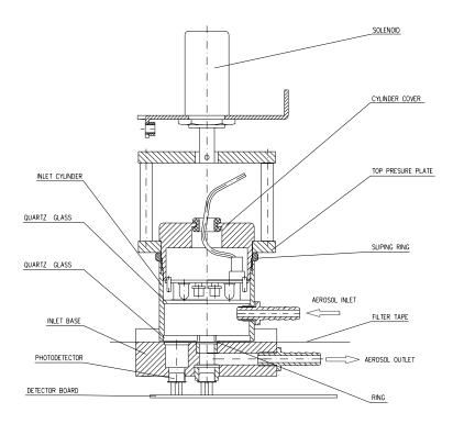
Figure 13: Cross-Section of Optical Analysis Head (diagrammatic only)
