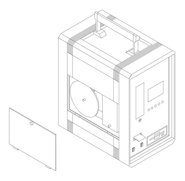
$\underline{\text{Figure 14}}$ : 'Portable' Aethalometer<sup>TM</sup> - left side front view, access door open
