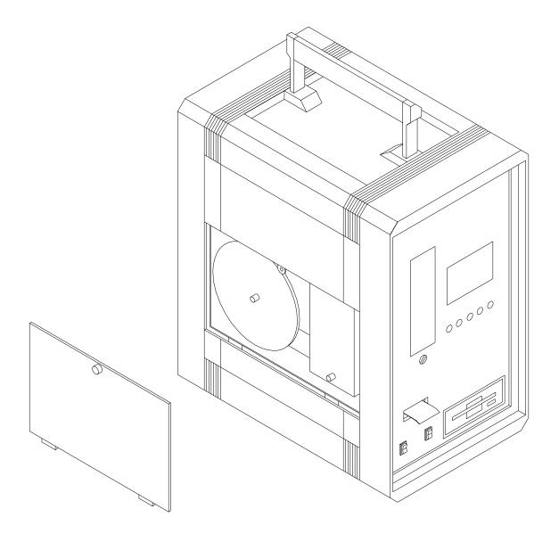
The Aethalometer TM - 'Portable' chassis version
