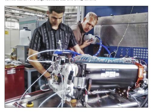
Figure 1: H<sub>2</sub>/O<sub>2</sub> polymer electrolyte fuel cell system developed in collaboration with Belenos Clean Power AG, Biel, Switzerland.
