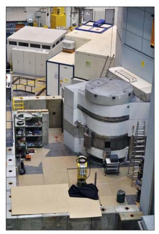
Figure 2: The EIGER area with the new monochromator shielding.
