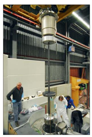
Figure 1: Insertion of the Deuterium moderator unit into the UCN vacuum tank. The moderator vessel, designed to contain up to 30 litres of solid Deuterium at 5 K, is located at the lower end of the unit.
