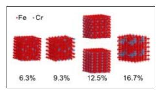
Figure 1: Representation of the lowest energy structures found for 6.3, 9.3, 12.5 and 16.7 at %Cr alloys.
