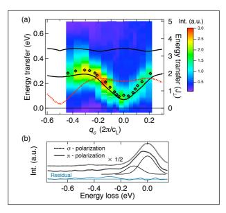
Figure 3: (a) RIXS data as intensity map vs. momentum and energy transfer. Calculated one-triplon (red dashed line) dispersion curve as well as the lower and upper border of the two-triplon continuum (black full lines) [5] are given for comparison. (b) RIXS spectra measured close to BZ centre for both linear polarizations. The  $\pi$  polarized spectrum can be fitted with two Gaussians; the residual is represented by the thin blue line.
