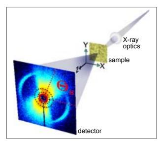
Figure 1: The experimental setup for scanning SAXS measurements. The sample is raster scanned through the focused X-ray beam and SAXS data are recorded at each point for the currently illuminated sample area. O₅ reveals the orientation of the illuminated nanostructure. A typical measurement comprises several tens of thousands of SAXS data frames recorded within half an hour.
