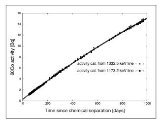
Figure 1: Activity of the two 60Co lines as a function of time.
