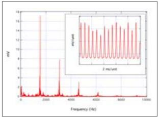
Figure 2: Bursts of coherent THz radiation appear in the beam spectrum at the synchrotron frequency of the low-a mode of 1.681 kHz. The inset shows the time signal. The current was 183 μA per bunch.
