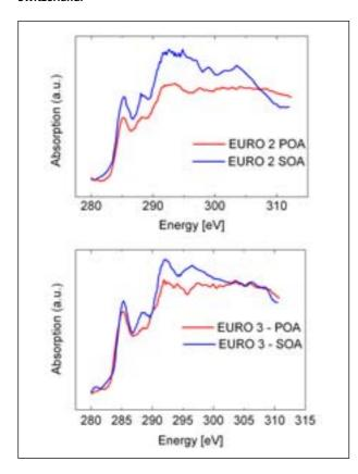
Figure 2: Carbon K-edge NEXAFS spectra of individual soot particles in samples taken immediately after injection into a smog chamber (POA, red) and after processing by simulated sunlight (SOA, blue). Results are compared for a Euro-2 (top) and a Euro-3 (bottom) diesel vehicle. The main features of interest are peaks at 285 eV (aromatic hydrocarbon species), 288 eV (carboxylic functional groups) and 292 eV (aliphatic hydrocarbons).
