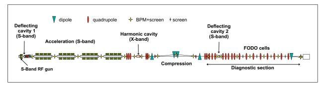
Figure 1: Schematic of the 250 MeV Injector test facility.
