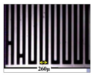
Figure 1: A magnified image of part of the SC wire.
