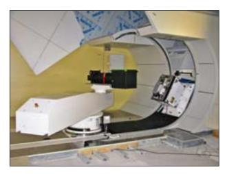
Figure 1: Gantry 2 area with table and nozzle.
