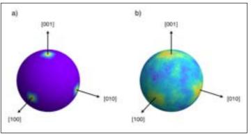
Figure 3: Spatial distribution of the H<sub>2</sub>O dipole moment of pure ice VII (left) and salty ice VII (right). In salty ice VII, the distribution is not strictly octahedral, and if dynamically distributed, is indicative of a plastic solid.
