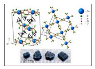
Figure 1: Crystal structure of Cu(pz)<sub>2</sub>(ClO<sub>4</sub>)<sub>2</sub> in a three-dimensional representation, and the projection onto the bc plane. The photograph shows the quality and size of the single crystals used in the experiments.
