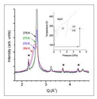
Figure: 1: Neutron diffraction patterns of LiCl:6D2O upon warming under 40 kbar pressure (see inset). Close to room temperature the amorphous sample (broad peak) crystallizes into salty ice VII (sharp peak). The tails around the main reflection peak are due to Huang scattering (see text). Reflection peaks marked with asterisks are from the pressure cell.
