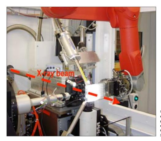
Figure 2: Sample-changing robot equipped with a gripper holding a crystallization plate into the X-ray beam at the X06DA beamline.
