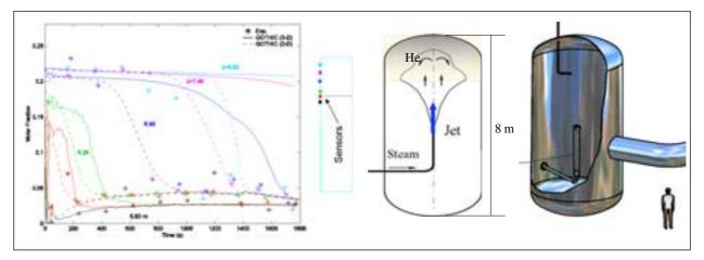
Figure 1: Simulation of a PANDA test with the GOTHIC code.
