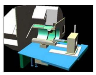
Figure 2: Patient positioning with sliding CT in the treatment area. The CT moves on rails.
