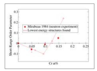
Figure 2: Weighted (1st and 2nd shell) short-range order parameter; full circles as measured by Mirabeau [5], empty circles as calculated for the lowest energy structures. The line is simply a guide for the eye.
