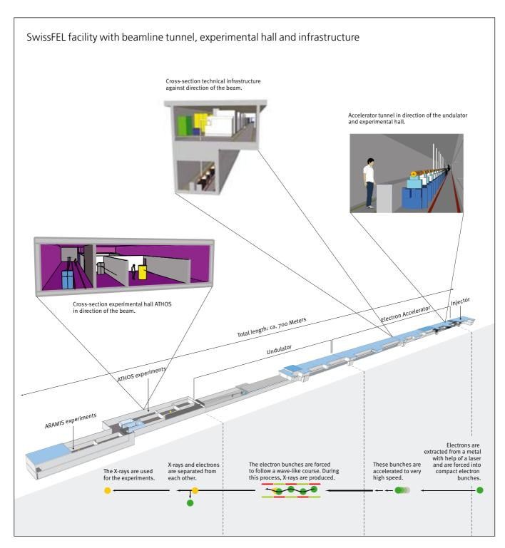
Figure 1: Schematic drawing of the SwissFEL.
