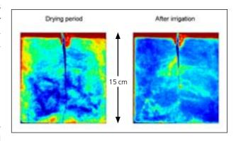
Figure 1: Neutron radiography of water distribution in a sample filled with a sandy soil and planted with a lupin. The pictures show the water content (blue = more water). Left: sample during the drying period, with more water around the roots. Right: sample after irrigation, with the rhizosphere dry.
