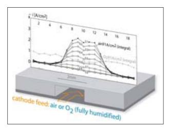
Figure 1: Direct measurement of local currents under channel and ribs of the flow field plate of a polymer electrolyte fuel cell (PEFC), in two operating modes.
