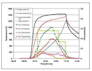
Figure 4: Experimentally measured temperatures and gaseous product mass flow rate during the solar steam-gasification of
