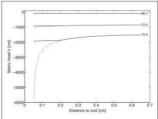
Figure 3: Calculated water potential near a root with (solid line) and without rhizosphere (dotted line). The rhizosphere weakens the drop in water potential that would occur in the case of a homogeneous soil, but favours root uptake as soil dries.
