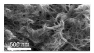
Figure 1: Scanning electron micrographs of a filtrated SWCNT material. The observed structures are bundles of several nanotubes. The diameter of a single nanotube is 1 - 2 nm.
