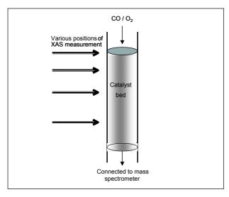
Figure 1: Plug flow reactor for in-situ XAS measurements.
