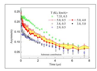
Figure 2: Muon decay asymmetry measurements versus time, with high (solid symbols) and low (open symbols) currents.
