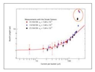
Figure 1: Bunch length as a function of current per bucket. The red full line is a fit of the empirical 3/8-power law to the data. For currents around 200 µA/bucket, the bunch length deviates from the empirical function as shown by the data points within the circle.
