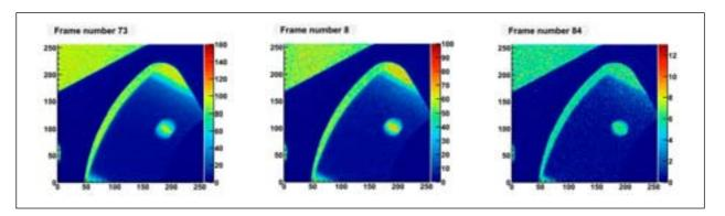
Figure 2: The blade of a rotating fan (100 Hz) recorded with 12bit counter depth, 125µs exposure time and 7.8kHz frame rate (left); 8bit counter depth, 85µs exposure time and 11.4kHz frame rate (center); and 4bit counter depth, 45µs exposure time and 20.8 kHz frame rate.
