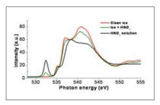
Figure 1: Surface-sensitive X-ray absorption spectra of clean ice, nitrate doped ice and HNO<sub>3</sub> solution.
