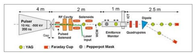
Figure 1: Schematic of the diode and RF cavity gun test stand installed at PSI.
