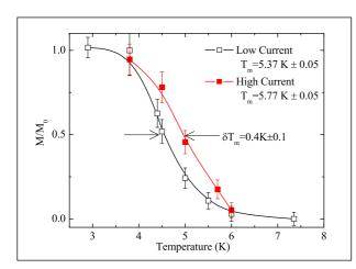
Figure 3: The magnetic phase transition with high (0.21c2) and low currents.  $M/M_0$  is the magnetic moment of the wire normalized to its low temperature value  $M_0$ . The solid lines are guides to the eye.
