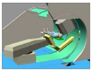
Figure 3: BEV: the mechanical system (in yellow) brings the flat panel from the parked position at the side of the nozzle to a position behind the patient.
