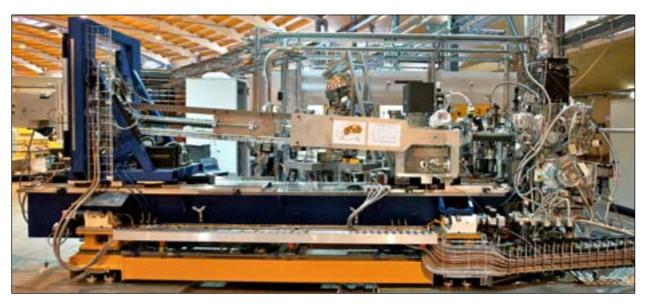
Figure 1: SAXES RIXS spectrometer at the ADRESS beamline.
