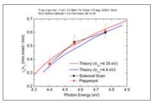
Figure 4: Intrinsic emittance per mm laser spot size (rms) versus the laser photon energy (Q < 1 pC, 5 MeV, 300 kV, 6 mm).
