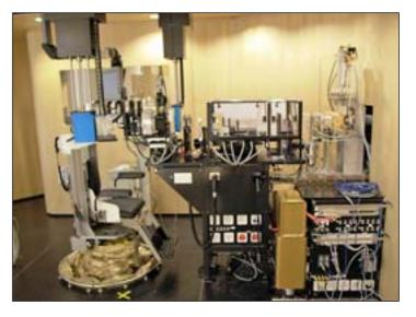
Figure 6: The OPTIS2 nozzle. The seat is mounted on a parallel robot and the blue squares are integrated flat panels used to position the patients using X-rays.
