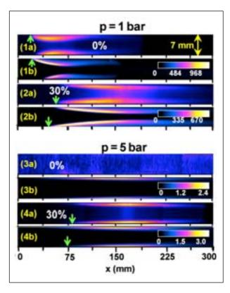
Figure 3: LIF measured (a), and numerically predicted (b), distributions of the OH radical during fuel-lean ( $\phi$  = 0.30) combustion of H<sub>2</sub>/air in a Pt-coated channel reactor with length 300 mm and height 7 mm. Cases (1) and (3) refer to no hydrogen pre-conversion, while (2) and (4) to 30% hydrogen pre-conversion. The arrows indicate the onset of homogeneous ignition. The bars provide the OH levels in ppmv.
