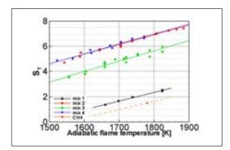
Figure 2: Turbulent burning velocity for hydrogen-rich fuel mixtures. Conditions: P=5bar, Tair = 673 K. Fuel mixture composition: #1 (H2-CO-CH4 20-20-60); #2  $(H_2\text{-CO }50\text{-}50); #3 (H_2\text{-CO }33\text{-}67); #4 (H_2\text{-CO-}N_2 40\text{-}40\text{-}20).$
