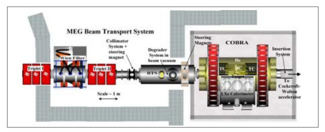
Figure 1: Schematic of the MEG experiment, showing the surface muon beam transport system, on the left, coupled to the superconducting COBRA positron-spectrometer and LXe photon detector. The drift chambers (DC) and timing-counter arrays (TC), as well as the thin target, are shown inside the COBRA magnet.
