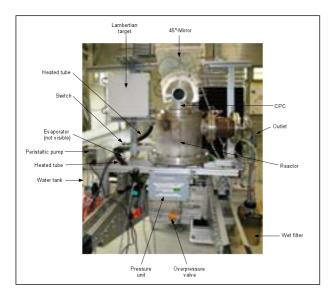
Figure 3: Photo of the 5 kW laboratory-scale solar gasification plant.
