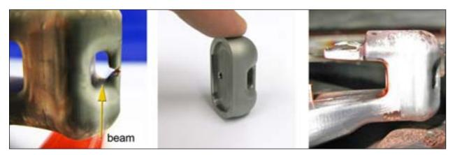
Figure 6: Damage of the puller nose due to loss of material by sputtering (left) has been decreased by applying a tungsten nose tip (middle) that does not show any degradation after 3 months of operation (right).
