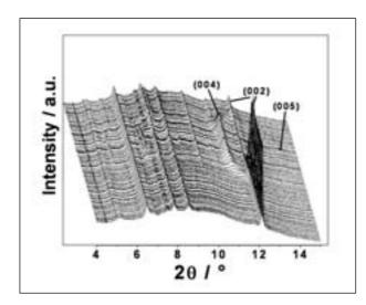
Figure 2: Synchrotron-based X-ray diffractograms (from bottom to top) recorded during a CV (3.0 - 5.2 V vs. Li/Li+) of SFG44 in EC:DMC 1:1, 1 M LiPF<sub>6</sub>.
