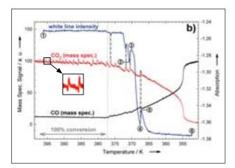
Figure 2: CO<sub>2</sub> and CO mass spectrometer traces plotted with the Pt L<sub>3</sub> white-line intensity measured in a plug flow reactor during the oscillating oxidation of CO.
