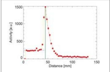
Figure 3: <sup>13</sup>N activity along the snow diffusion chamber as measured by the coincident γ-counter during exposure of the snow sample to HO13NO. The solid line at 45 mm represents the gas/snow interface.
