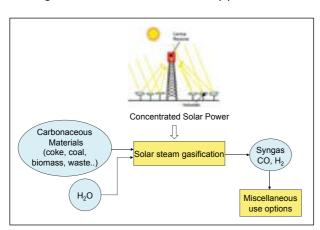
Figure 1: Scheme of solar steam gasification.
