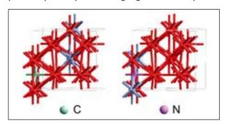
Figure 3: 2×2×2 supercells with 14 Fe, 2 Cr and either 1 C or 1 N.
