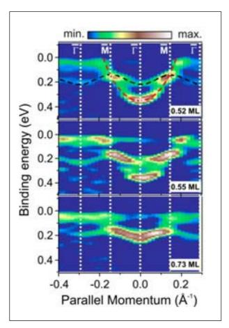
Figure 2: Angle-Resolved Photoemission Spectra (2<sup>nd</sup> derivative) depicting the distribution of electronic states in a surface, dependent on the surface coverage of the porous network. The red and black dashed lines in the uppermost image indicate the averaged positions of the maxima of both Lorentzian components fitted for all measurements.
