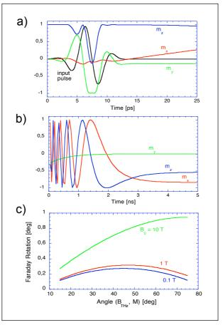
Figure 3: Simulated magnetic switching induced by a 6 T THz pulse in a permalloy film at short (a) and long (b) times. c): Faraday rotation angles predicted for THz signals of various amplitudes upon transmission by a 600 nm film, as a function of the initial polarization direction.
