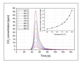
Figure 3: Cathode exhaust gas CO<sub>2</sub> concentration as response to a triangular potential pulse between 0.6 and 1.3 V for different cell temperatures (fully humidified gases). The inset shows the resulting carbon corrosion rates, which are obtained by integration of the CO<sub>2</sub> peak areas.
