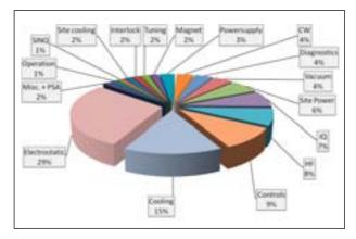
Figure 2: **Downtime** characterization for outages in the p-facility longer than 5 minutes (ca. 340 hours).
