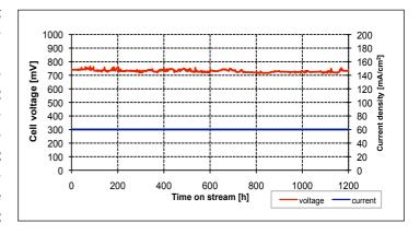
Figure 3: Results of a long-duration test with a tubular SOFC run with wood gas at PSI [2].
