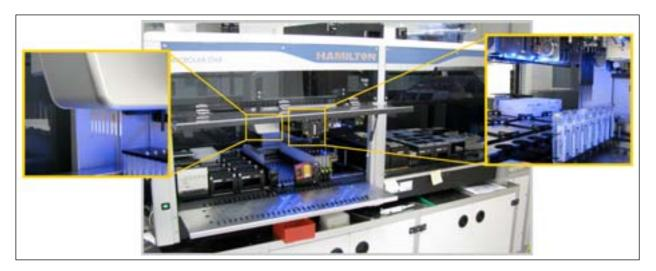
Figure 1: Liquid-handling robot of the crystallization facility. The platform can carry out all steps of the workflow necessary to set up crystallization experiments in the nanolitre scale.
