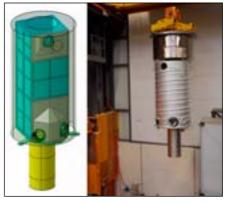
Figure 2: Finished setup of the UCN storage volume surrounded by the heat radiation shield, vertical UCN auide on the bottom and ~10 tons steel shielding on top (about 5m tall): a) design drawing, b) during transport to its final position in the UCN tank.
