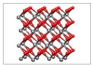
Figure 2: UO<sub>2</sub> (U grey, O red) fluorite structure at 0 K.
