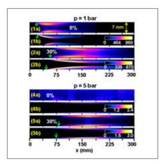
Figure 3: Distributions of the OH radical: measured by LIF (a), and numerically predicted (b).  $\varphi = 0.30$ , H<sub>2</sub>/air, Pt coating. Cases (1) and (3): no hydrogen pre-conversion; (2) and (4): 30% H<sub>2</sub> pre-conversion. Arrows indicate onset of homogeneous ignition. Colour code: OH level in ppmv.
