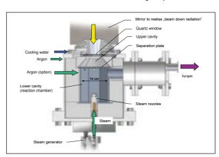
Figure 2: Scheme of the solar reactor configuration.
