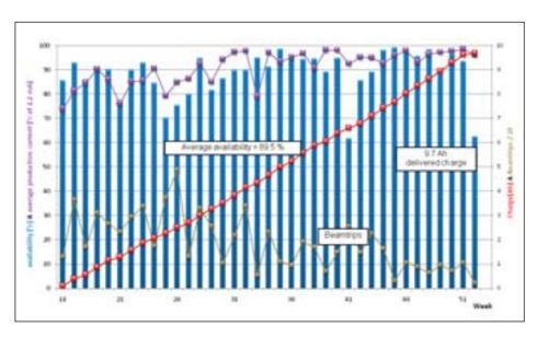
Figure 3: Operation of the Proton Facility: availability, average current, delivered charge and beam trips.
