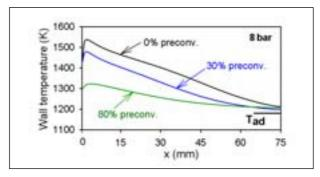
Figure 4: Computed wall temperature profiles in a catalytic honeycomb reactor. Pt coating, p = 8 bar.  $\phi = 0.30$ ,  $H_2$ /air, three different pre-conversion ratios. adiabatic equilibrium temperature  $T_{ad} = 1181 \text{ K (for all cases)}$ .
