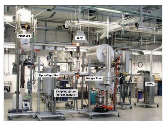
Figure 1: Flexible set-up for long-duration tests of B-IGFC concepts, including gasifier, gas cleaning and high-temperature fuel cells.
