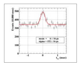
Figure 2: Measured coincidence time spectrum tey at normal beam rate, showing the RMD peak above the accidental background and the fitted resolution function.
