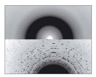
Figure 2: Comparison of XRD data for ettringite (spot 1 in Fig. 1) collected with beam sizes of 200  $\times$ 100  $\mu m^2$  (top) and 10  $\times$  10  $\mu m^2$ (bottom).
