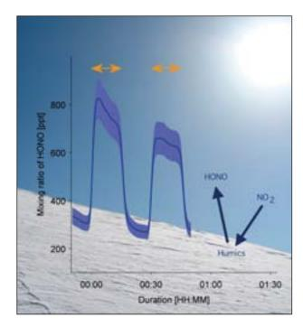
Figure 2: Evolution of the HONO gas phase mixing ratio with time (solid line) after contact with humic acid doped ice. Two consecutive irradiation periods in the visible range (orange arrows) in the presence of NO2 in the gas phase are shown. The shaded area illustrates the accuracy of the HONO measurement. Time zero denotes the beginning of the (first) irradiation period.
