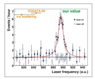
Figure 1: Resonance curve of the 2S-2P transition in muonic hydrogen. On resonance, we have measured a rate of 6 events per hour. The line position predictions (in orange) have been computed using the proton radius values given in [3] and [4].
