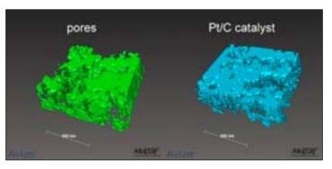
Figure 4: 3D images of a PEFC active layer – pore structure (left) and carbon supported catalyst (right). Images were segmented and reconstructed from SEM images, obtained during FIB/SEM serial sectioning of a commercial PEFC cathode.
