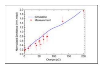
Figure 3: Normalized projected emittance at 5 MeV (6 mm gap, 300 kV pulser voltage, 6.72 A/mm<sup>2</sup> current density, 4.2 ps (rms) laser duration).
