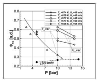
Figure 1: Operational window for a fuel mixture of 50% H<sub>2</sub>/50% CO.
