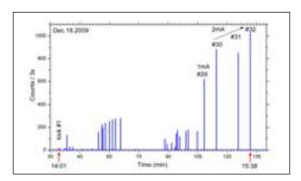
Figure 1: Observed neutron counts in the experimental West area during beam testing. Neutron counts peaked at times, unambiguously matching proton beam kicks. The detected neutron intensities were found to depend on proton beam current and tuning.
