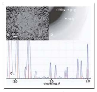
Figure 3: Characterization of a C-S-H-area of the alteration zone: a) SEM image; b) micro-diffraction pattern and c) one-dimensional diffraction diagram of 11 Å tobermorite. Diffraction lines shown in red were predicted from the structure.
