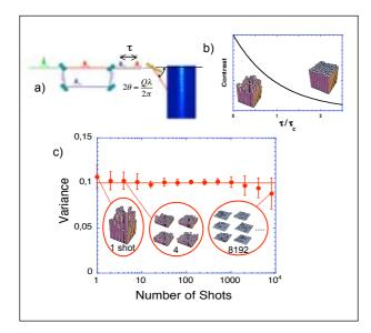
Figure 2: With split-pulse XPCS (a), the Q-dependent correlation time of a system is determined via the speckle contrast (b). Simulations (c) demonstrate an optimum number of shots and the usefulness of very sparse data.
