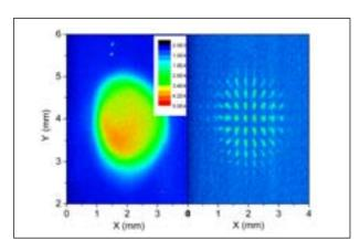
Figure 2: Measured electron beam transverse profile and corresponding pepper-pot picture (13 pC, 5.1 MeV, 0.23 mm.mrad).
