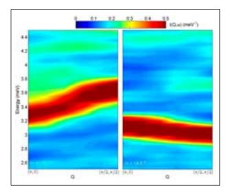
Figure 2: Zone-boundary excitations, showing a dispersing long-lived excitation and a continuum for wave-vectors  $(\pi,0)$ in  $Cu(pz)_2(ClO_4)_2$ .  $(\pi,0)$  corresponds to wave-vectors along the square edges, while  $(\pi/2,\pi/2)$  to diagonal wave-vectors.
