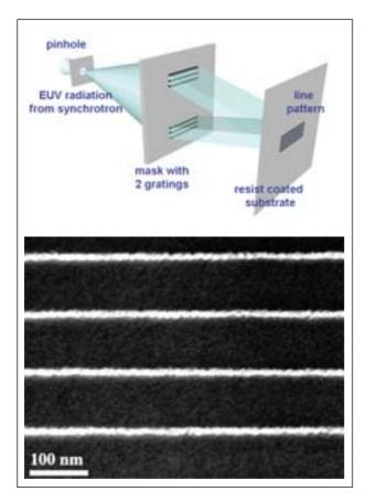
Figure 2: The EUV-IL station installed at the SLS uses holographic grating masks for ultra-high-resolution exposures in the EUV range (top).
