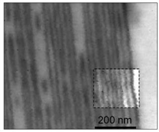
Figure 2: Scanning X-ray microscope image of a test object consisting of lines and spaces down to 15 nm in width. Photon energy: 1 keV.
