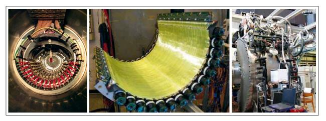
Figures 2 (Left): – COBRA central He-volume, with the Drift Chamber Assembly including the mounted target. The beam entrance window can be seen at the far end (Centre): – Timing Counter assembly with scintillating fibres and APD readout exposed (Right): – Liquid Xenon (LXe) Calorimeter installed in the πE5 area
