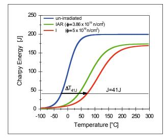
Figure 1: Charpy energy vs. temperature for un-irradiated, irradiated (I), and irradiated-annealed-re-irradiated (IAR) specimens [2].
