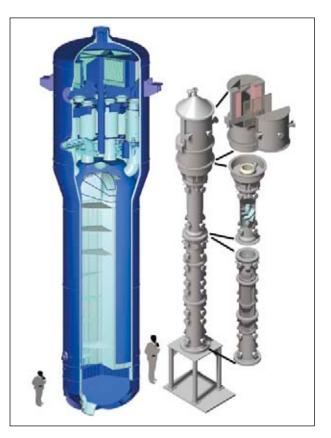
Figure 1: Schematic of the KKB SG alongside the ARTIST facility showing the relative proportions.
