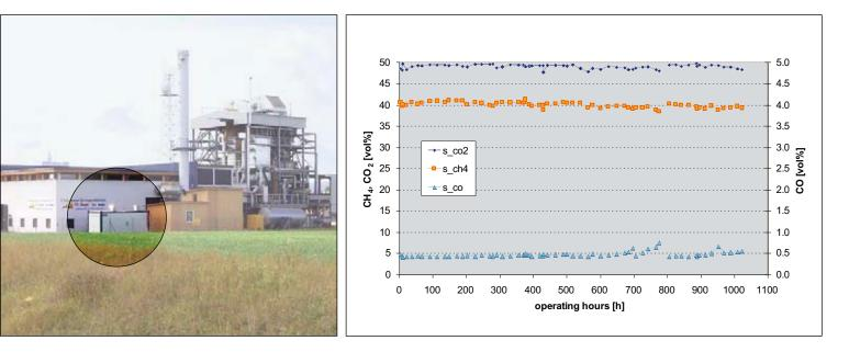
Figure 1: PSI 10 kW scale test facility (inside white container) at the industrial wood gasifier in Güssing/Austria (left), concentrations of methane and carbon oxides during the 1000h test (right)
