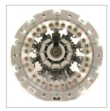
Figure 1: Prototype detector assembly for ALC µSR, equipped with Avalanche Microchannel Photodiodes (AMPD's) tested in magnetic fields up to 5 Tesla.
