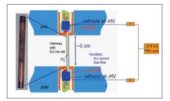
Figure 3: Schematic view of the proton source in the cyclotron center. Free electrons, created in arcs between cathodes and anodes, are trapped in the chimney and ionize gas that is flushed into the source. The protons can leave the chimney though a slit and are pulled towards the first HF electrode.
