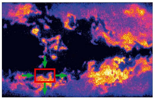
Figure 1: The combination of laser induced fluorescence with particle induced velocimetry provides access to the local heat balance. In developing methods for the efficient, low NOx combustion of synthesis gas, this information is important to assess flame stability and to suppress thermoacoustic oscillations.
