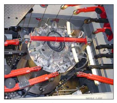
Figure 1: The shielding flask and sample changer on top of the PROTEUS reactor
