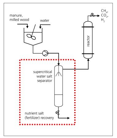
Figure 1: Schematic representation of PSI's catalytic hydrothermal gasification process (excluding heat exchangers and gas/water separation).
