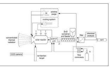
Figure 2: Experimental set-up of the solar reactor and peripherals at PSI's High-Flux Solar Simulator.
