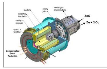
Figure 1: Schematic of the solar chemical reactor configuration.
