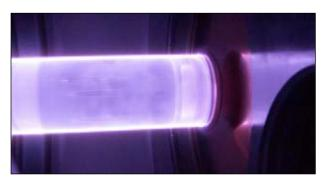
Figure 2: Glow discharge, used for high-voltage, high-gradient commissioning of the 500 kV pulser.
