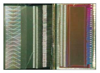
Figure 1: Pixel array of profile monitor (left) with bond wires (centre) and APC128 read-out chip.
