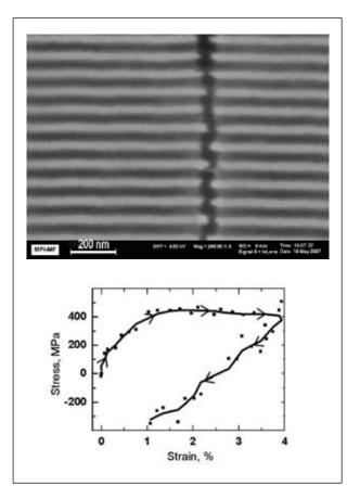
Figure 3: a) SEM image of Au nanowires on polyimide substrate. First cracks perpendicular to the loading direction appear at a strain of 2.4%, b) Stress/strain curve of Au nanowires with 20 nm height and 50 nm width in loading direction. The arrows show the strain change direction. The yield stress averages approximately 400 MPa which is one order of magnitude higher compared to the yield stress of bulk gold and the same as in a corresponding thin film.
