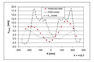
Figure 4: Comparison between CFD and measured velocity data.
