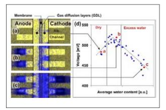
Figure 1: *In plane* Neutron Radiograms (2.5 µm per pixel perpendicular to membrane) of a PEFC showing the water distribution at 1A/cm<sup>2</sup> for different inlet relative humidities at the anode/cathode: (a) 60%/0% (b) 110%/40% (c) 90%/ 110%.
