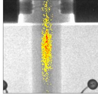
Figure 3: Snapshot of the distribution of  $H_2O$  injected as a tracer pulse into the high pressure separator filled with  $D_2O$  (400 °C, 30 MPa; 1 s shutter time).
