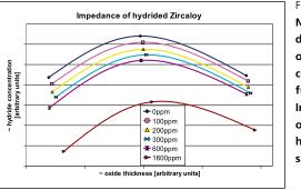
Figure 1: Non-destructive determinations of hydride concentration in fuel claddings: Impedance curves of differently hydrided zircaloy samples.
