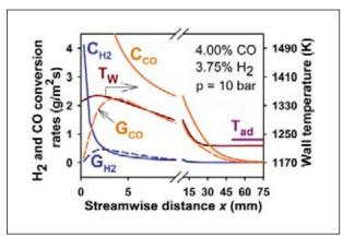
Figure 2: Computed profiles of catalytic (C) and gas phase (G) conversion rates of  $H_2$  and CO, and surface temperature ( $T_w$ ). Inlet temperature: 600 K. Tad: adiabatic equilibrium temperature.
