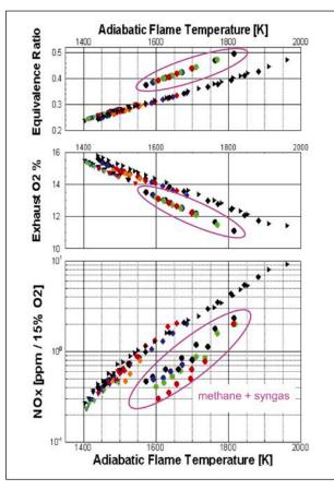
Figure 1: NO<sub>x</sub> emission and operational range for all investigated syngas mixtures at several conditions.
