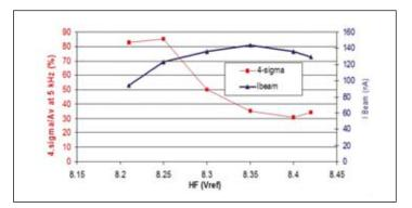
Figure 4: HF voltage effect on intensity and stability.
