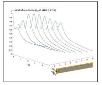
Figure 3: Locally resolved (9 segments, 63 cm<sup>2</sup> active area) transient response of the hf resistance (5 kHz) in a nine-fold segmented PEFC with linear flow field, after a stepwise increase in current from 0.1 to 0.8 A/cm<sup>2</sup>.
