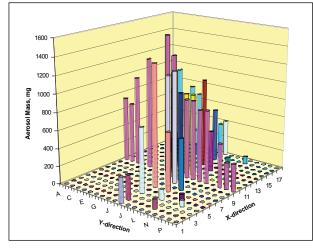
Figure 2: Aerosol deposition profile in the tube bundle.
