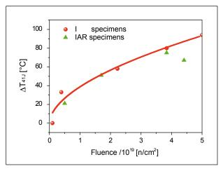
Figure 3: The shift  $\Delta T_{41J}$  of the transition temperature vs. fluence for the I and IAR specimens.
