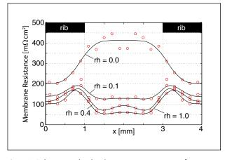
Figure 2: *Sub-mm* resolved resistance measurements of membrane under channel and rib at different relative humidity (rh). Current density 400 mA/cm<sup>2</sup>; Tcell = 70 °C; p = 1.5 bar<sub>a</sub>.
