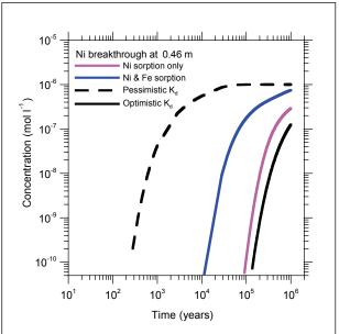
Figure 3: Calculated Ni<sup>2+</sup> concentration at the bentonite buffer/ host rock interface. Sorption of Ni(II) is described by multispecies reactive transport, including mechanistic sorption models. A second calculation accounts for the effects of sorption competition between Ni and Fe. The results from calculations based on the simple K<sub>d</sub> approach using bounding pessimistic and optimistic K<sub>d</sub> values for Ni(II) are also shown.
