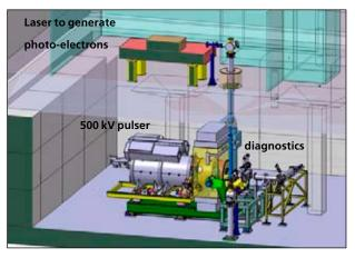
Figure 3: Layout of the present electron source. See text for details.
