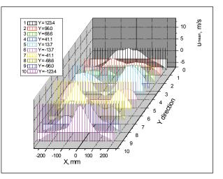
Figure 3: Vertical velocity profiles in the tube bundle.
