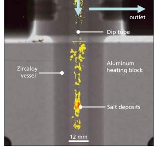
Figure 2: Build-up of solid Na<sub>2</sub>SO<sub>4</sub> around the dip tube inside the separator, finally leading to a vessel blockage (405 °C, 30 MPa; Feed: Na<sub>2</sub>SO<sub>4</sub> + Na<sub>2</sub>B<sub>4</sub>O<sub>7</sub> in D<sub>2</sub>O; 15 s shutter time).
