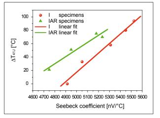
Figure 4: Correlation between  $\Delta T_{41J}$  and the Seebeck coefficient for the I and IAR specimens.
