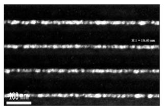
Figure 1: SEM image of 10 nm wide Au lines obtained with EUV-IL and novel lift-off processes.
