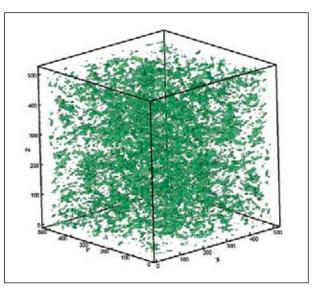
Figure 2: Entropic Lattice Boltzmann simulation of the three-dimensional Kida-vortex flow at Re=20000. Iso-vorticity surfaces at the peak of enstrophy are presented on a 512 x 512 x 512 grid.
