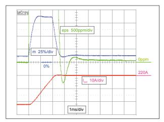
Figure 1: U-sweeper closed loop control performance.
