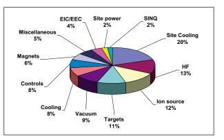
Figure 2: Downtime characterization for interruptions llasting more than 10 minutes (ca. 300 hours).
