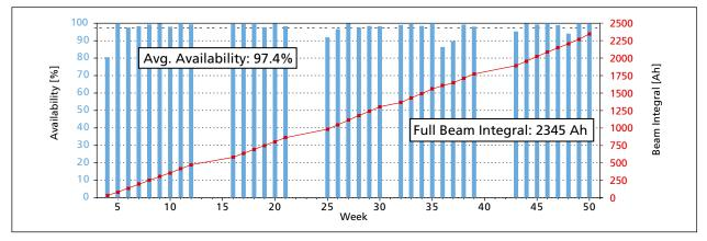
Figure 1: SLS operation statistics: weekly availability and integrated beam dose.
