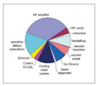
Figure 2: The subsystems causing unscheduled down time in 2007.
