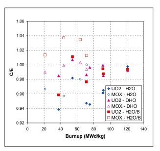
Figure 2: Calculated-to-experimental (C/E) ratios for the reactivity worths of the burnt samples vs. burnup (DHO =  $D_2O/H_2O$  mixture, H2O/B = borated H<sub>2</sub>O)
