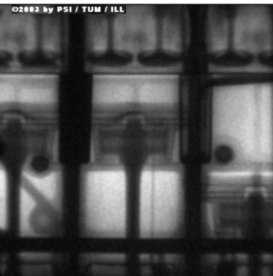
Figure 4: Technische Universität (TU) München, Institut Laue-Langevin (ILL) Grenoble and PSI: sequence of oil lubricant distributions inside a running 4-stroke combustion engine.
