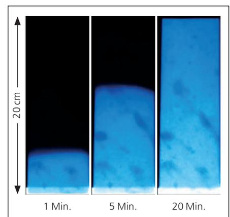
Figure 2: **Study of the water absorption of limestone over a range of 20 minutes and the determination of specific diffusion properties, snapshots of one series of measurements.**
