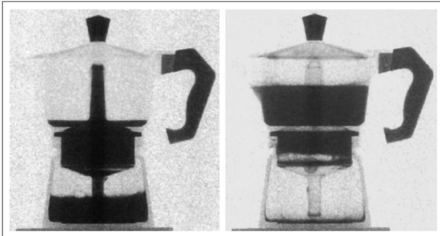
Figure 3: Coffee pot and boiler, two-phase flow of water and vapour inside the metallic structure, frame rate of 25 pictures/sec, "real time" flow monitoring.
