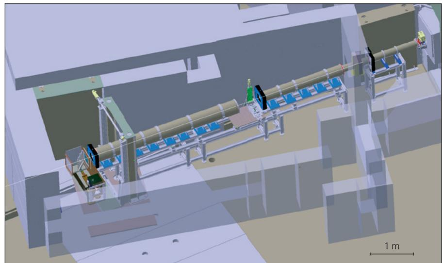
Figure 1: **Layout of the neutron imaging facility ICON at the Spallation Neutron Source, SINQ: two different beam positions offer a wide dimensional range for samples or engineering installations.**
