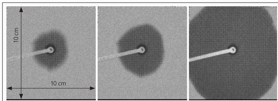
Figure 5: Time-dependent sequence of the penetration of liquid polymer resin in woven glass fibre fabric over a range of a few seconds, 2D recording of the impregnation process and visualization of the anisotropy of the textile structure.
