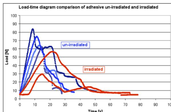
Figure 2: Comparison of unirradiated and irradiated adhesive bonds.
