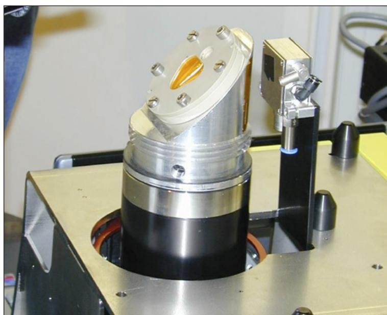
Figure 5: Specimen holder for radioactive samples to be investigated at the Swiss Light Source, SLS.
