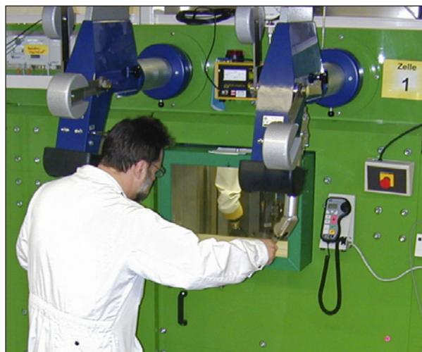
Figure 1: Integration of a universal testing machine in a completely shielded  $\alpha$ -radiation-proof box.
