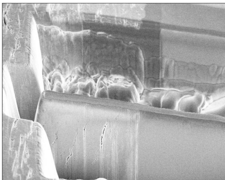
Figure 4: Intersection of a sample at the interface of a zirconium alloy and its oxide (width 20 µm).
