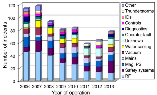
Figure 6: Beam outage count per failure category
