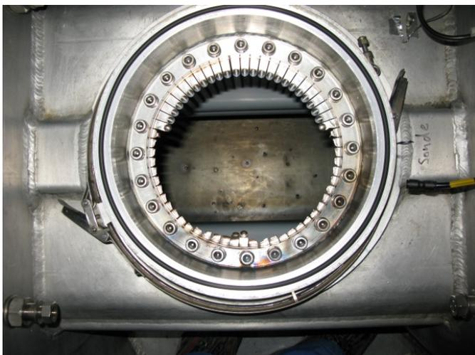
**Figure 3:** Burned finger contacts at the RF entrance of the ring flattop cavity
