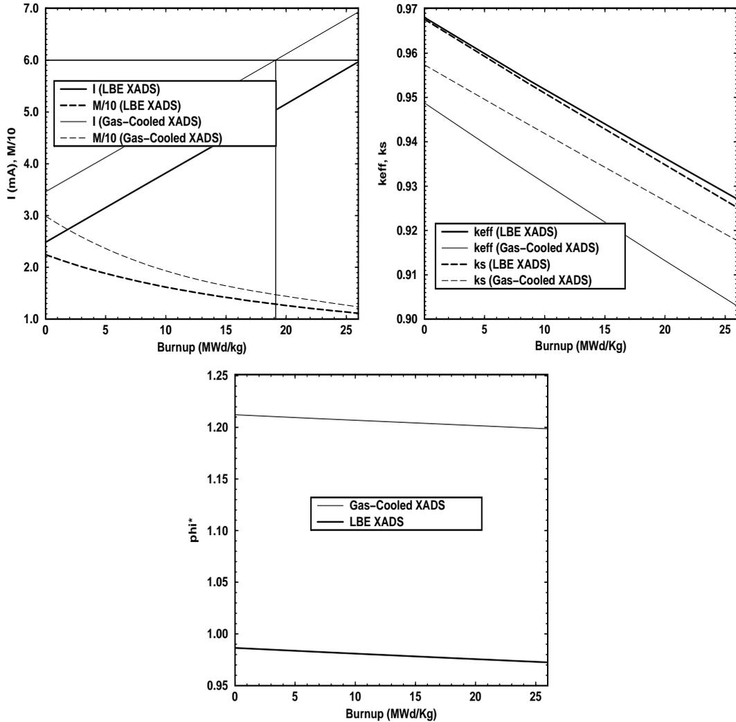
**Fig.1** Beam current ( $I$ ), normalised number of fission neutrons ( $M/10$ ), multiplication factor (“ $k_{eff}$ ”), source multiplication factor (“ $ks$ ”) and source importance (“ $\phi_i^*$ ”)
