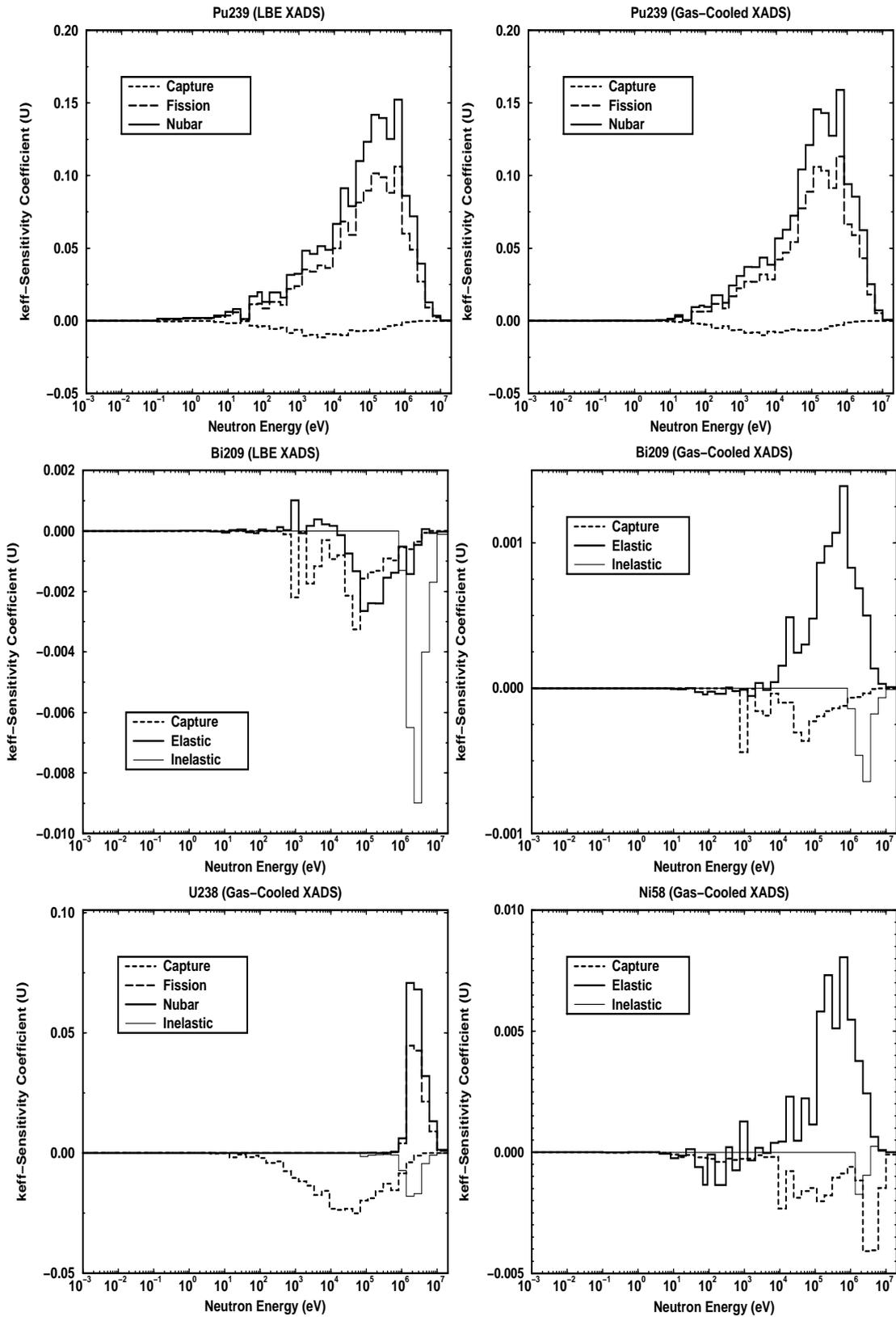
**Fig.2** Sensitivity profiles of  $k_{eff}$  due to important nuclides and reactions
