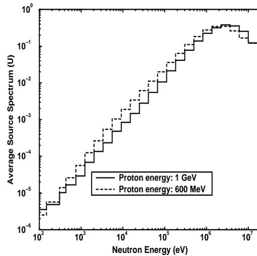
**Fig.3** Average energy spectra of the external neutron source
