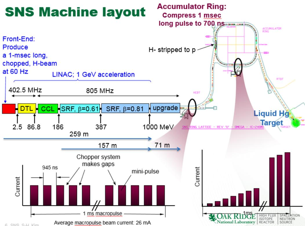
Figure 12: The SNS linac layout and the beam time structure.
