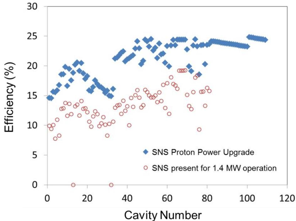
Figure 15. Efficiency comparison of individual SRF cavities between the present setup for 1.4-MW operation and the Proton Power Upgrade (plan) for 2.8-MW operation.
