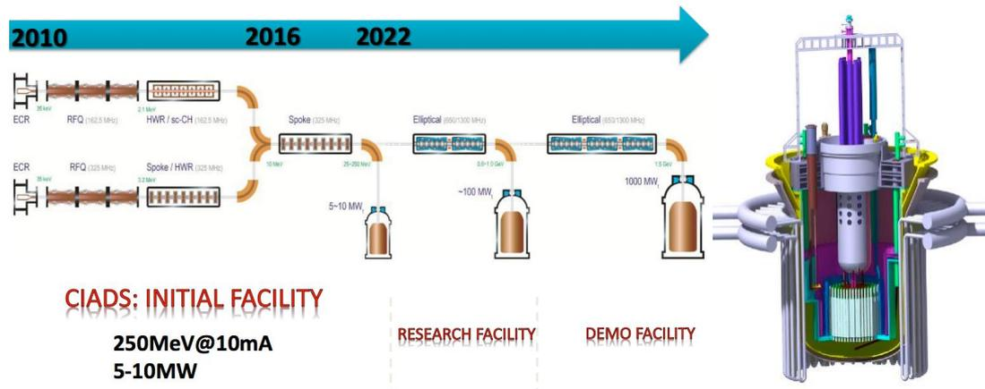
**Figure 2: Chinese Accelerator Driven Advanced Nuclear Energy System (ADANES) project with two parallel injectors, the target and the blanket (on the right) proposed as a complete energy system integrating nuclear waste transmutation and energy production (Physics 2016 Vol. 45 (9): 569-577).**
