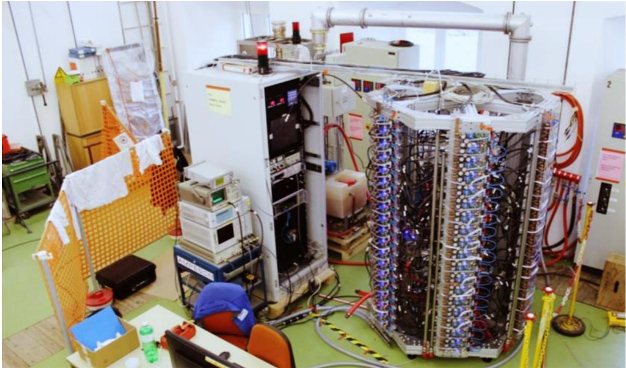
Figure 6: 65 kW, 500 MHz solid state amplifier at PSI (Marcos Gaspar, PSI).
