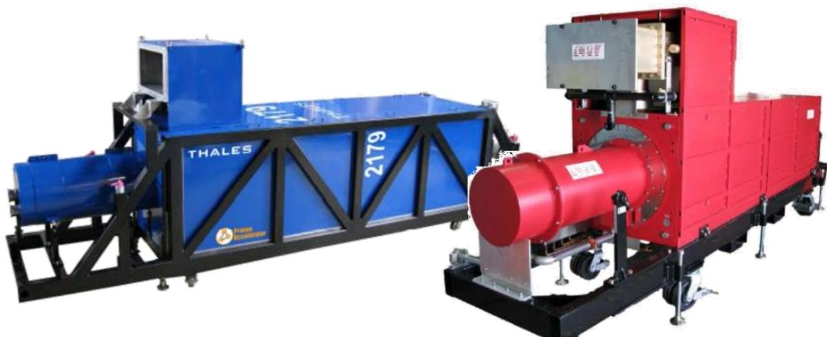
Figure 5: 352 MHz klystrons by Thales and CPI as used in Linac4 and foreseen for the ESS warm linac (Chris Lingwood, Lancaster University).
