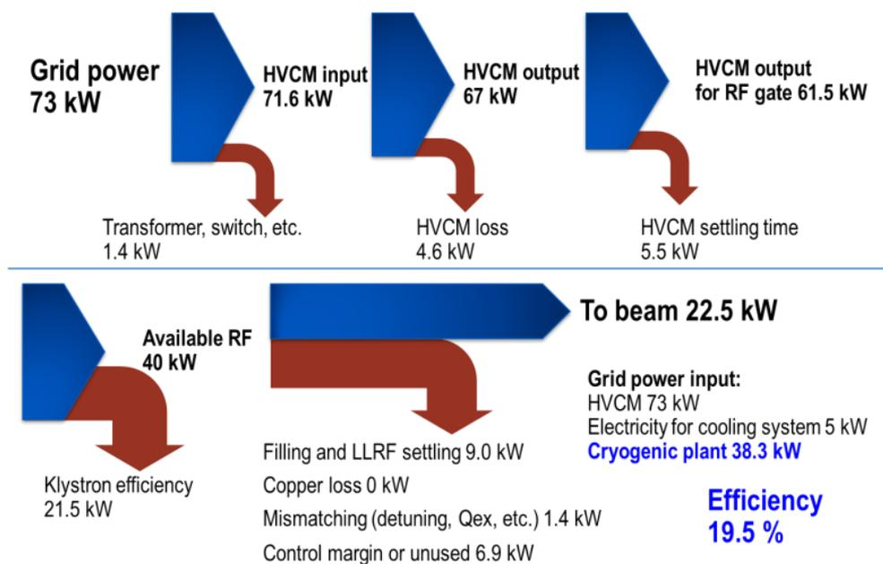
Figure 14: Example of power flow of a SRF cavity.
