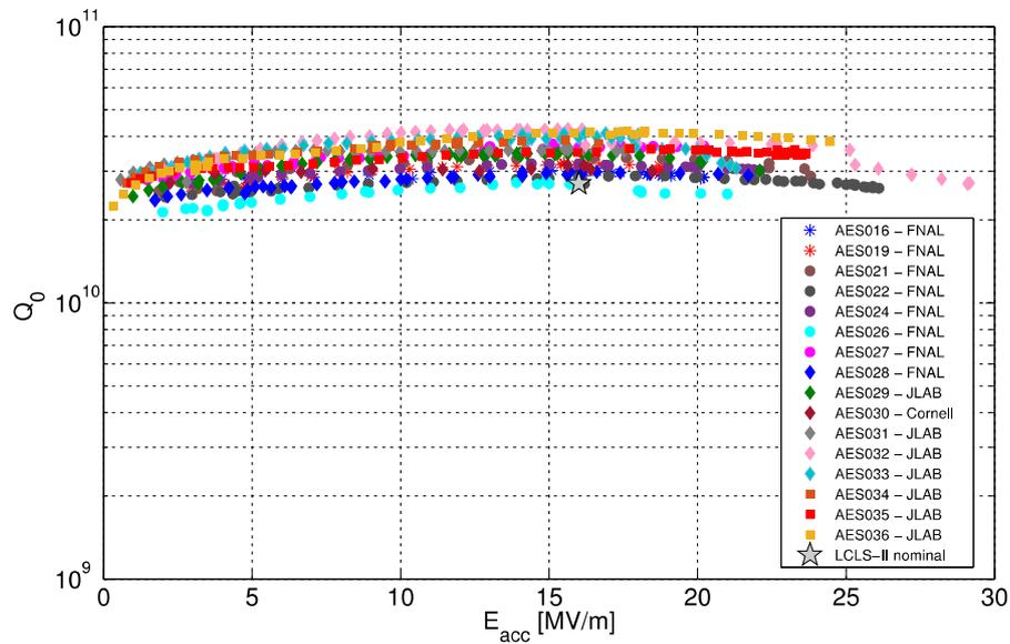
Figure 19.  $Q_0$  versus the acceleration gradient for dressed LCLS II cavities (A. Grassellino).
