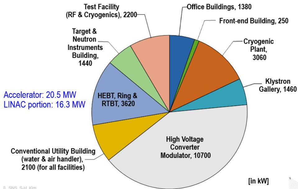
Figure 13: Power consumption breakdown of the spallation neutron source (SNS)
