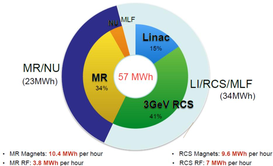
Figure 18. The power consumption diagram for J-PARC accelerator facility.
