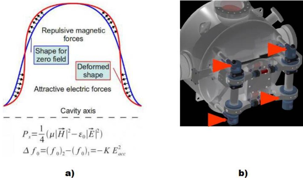
Figure 20: a) Lorentz Force Detune (LFD) mechanism, and b) piezo tuner for LFD and microphonics mitigation.
