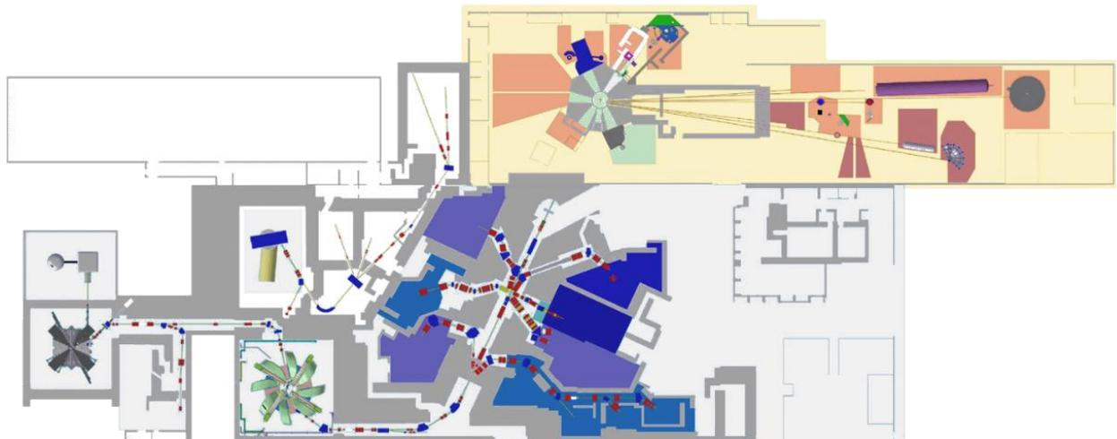
Figure 10: PSI cyclotron facility layout showing Muon beamlines and the neutron source with instruments in the upper part of the graphics.
