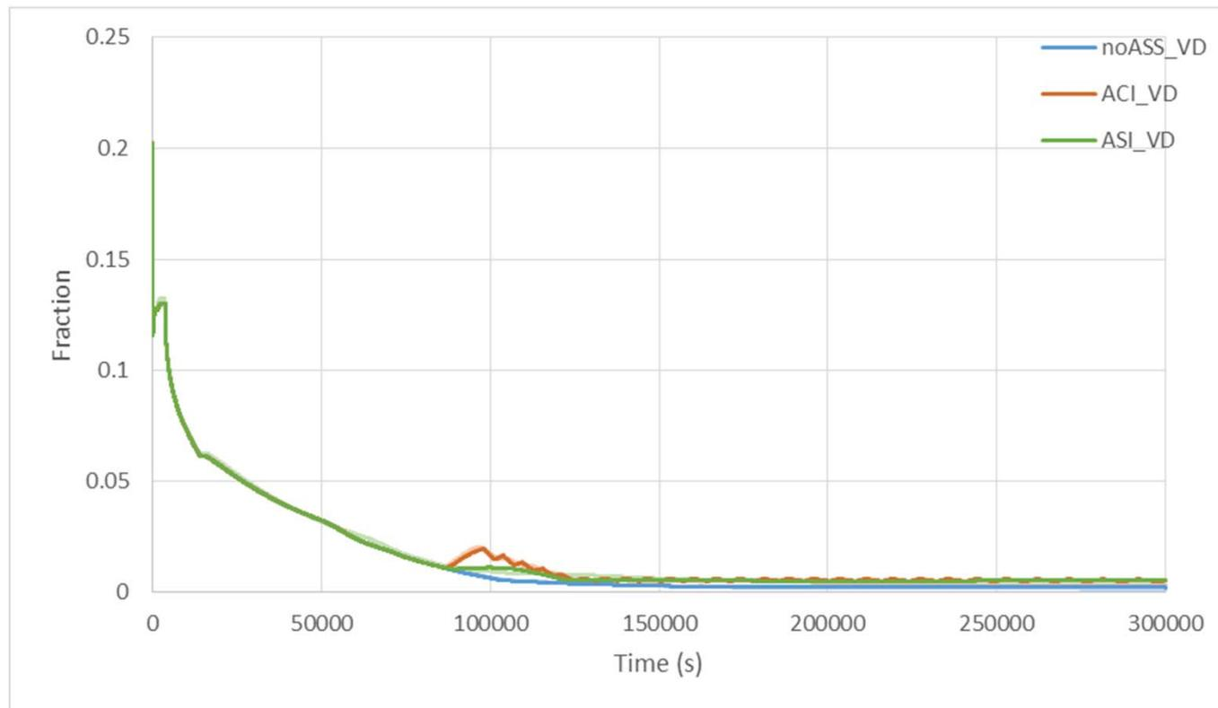
O<sub>2</sub> fraction is in general low due to oxidation processes (mainly due to PARs operation)
