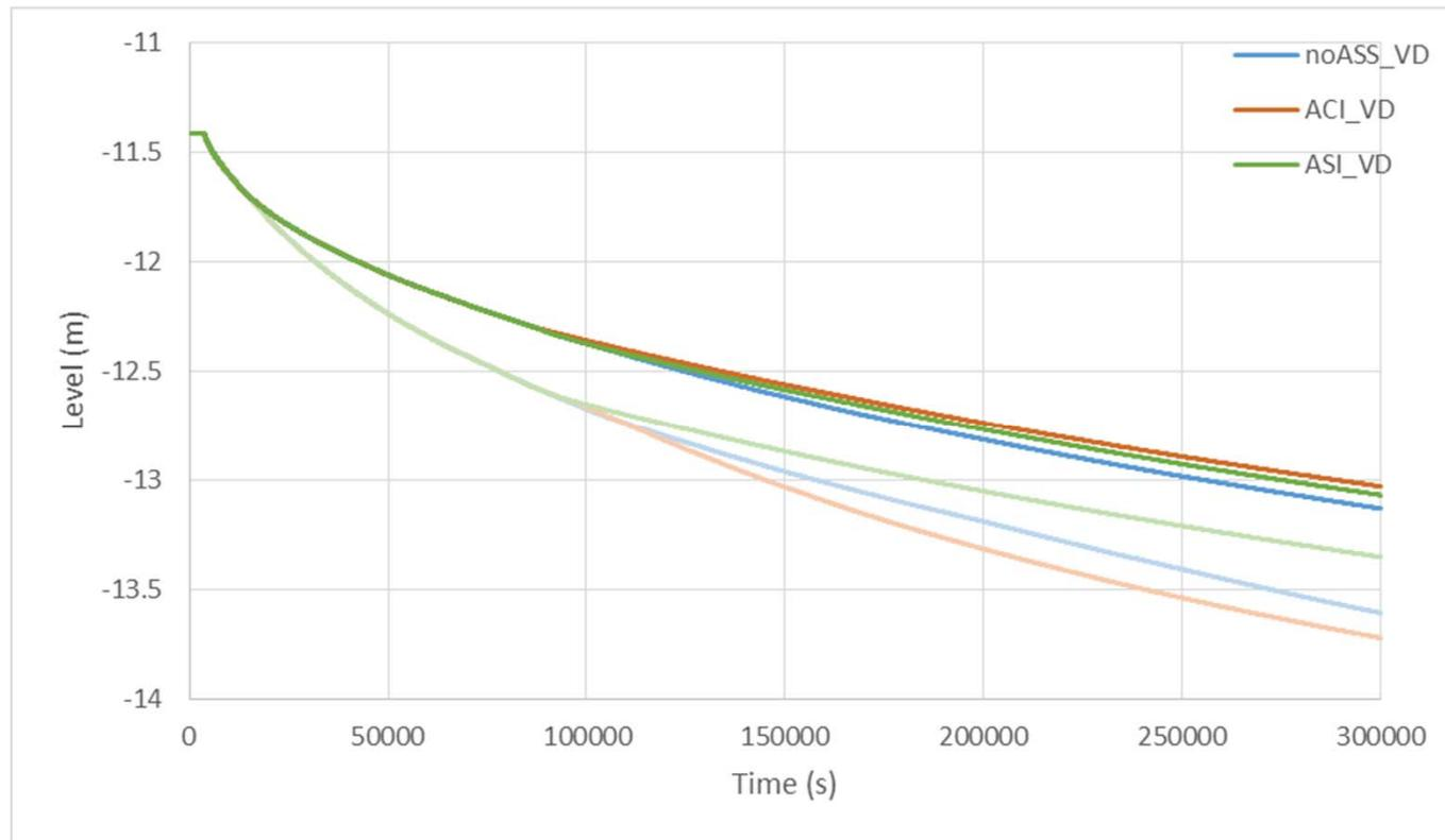
Natural circulation with VD: improved heat transfer from melt to containment atmosphere
