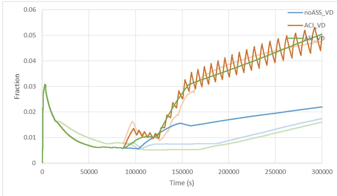
Global H<sub>2</sub> fraction is typically below 5% limit for combustion due to PARs
