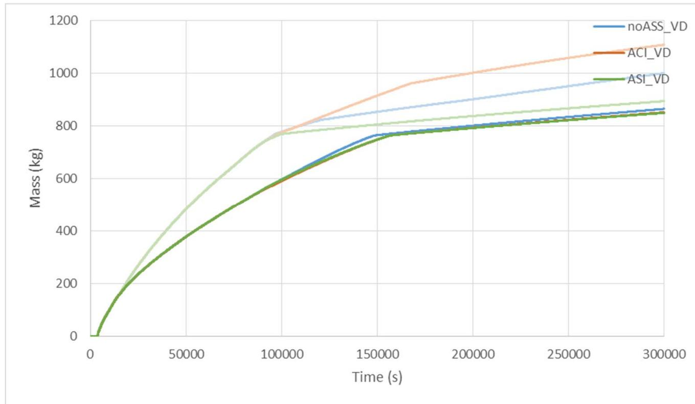
In-vessel about ~170 kg H<sub>2</sub> is released
