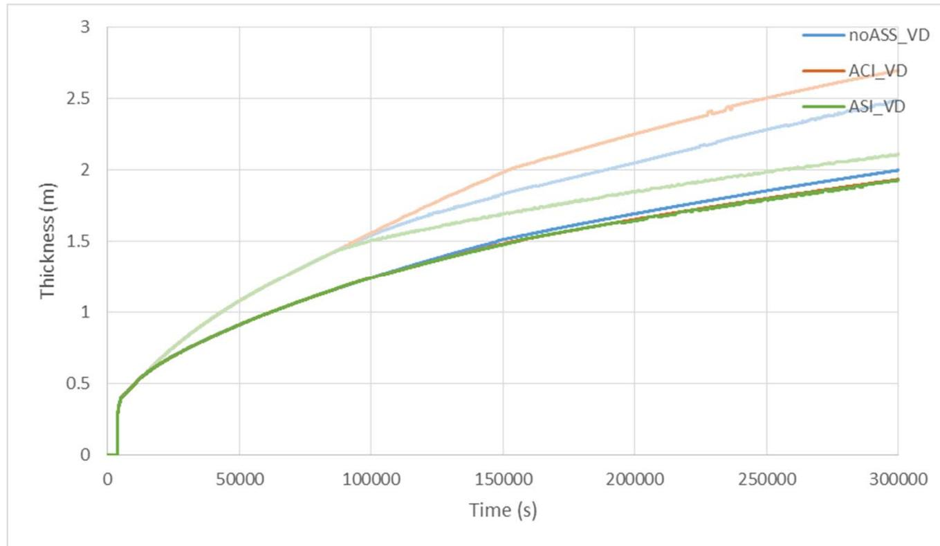
By heat conduction through corium crust only ~8 cm thick melt layer may be cooled
