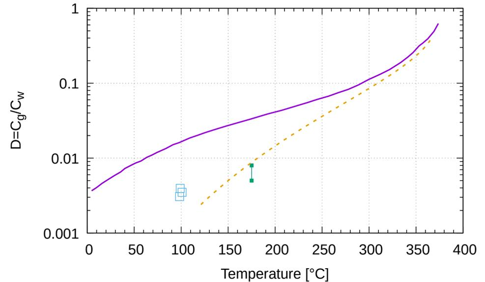
Pool→steam distribution coefficient  $D$  in boiling conditions.
