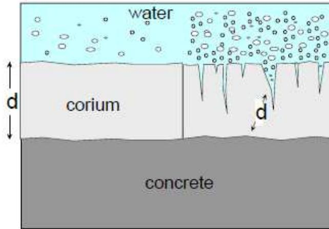
Corium Crust to Water Heat Flux
