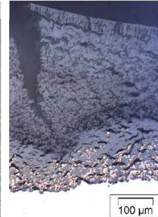
Zry-4 cladding oxidation for 1 hour at 1000°C in air
