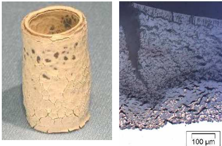
Zry-4 cladding oxidation for 1 hour at 1000° C in air
