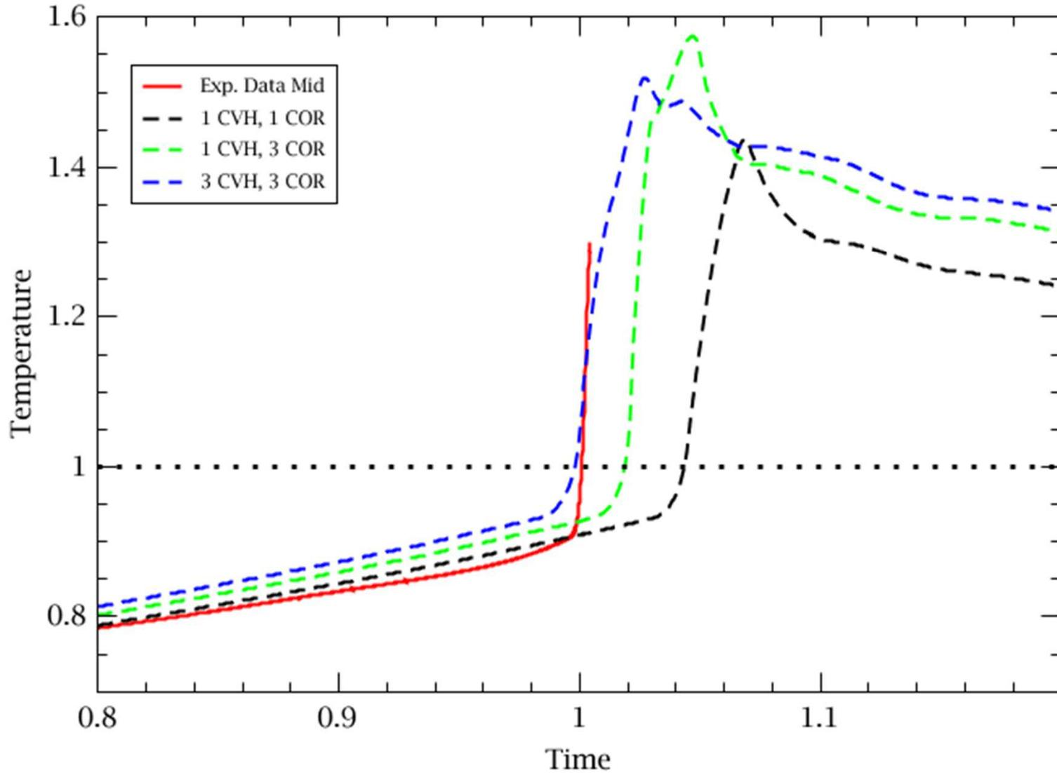
At several elevations of the fuel bundle temperature profiles were measured at different rods. From this data a radial temperature distribution could be deduced. Comparison of the calculated data of the 3 radial nodes showed a surprisingly good estimation with the experimental data. The “plane” of the measured data is slightly below the “plane” of the calculated data and therefore a shift is observed due to the slowly downward propagation of the zirconium fire.
