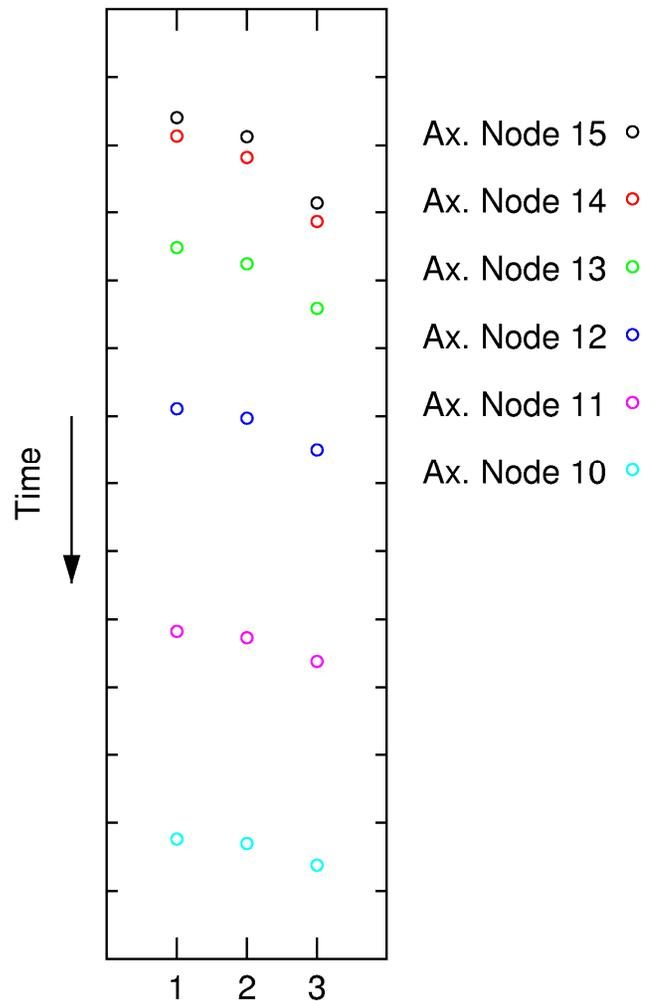
The crust breakup signals for the different radial nodes are the starting signals for the heatup leading to ignition of the zirconium fire. As can be seen, the ignition started in the upper region of the fuel element and then the zirconium fire propagates downward.
