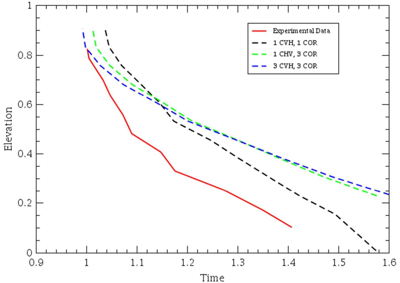
The downward propagation velocity of the zirconium fire is very closely reproduced by the MELCOR calculation for the simplest geometrical model with only 1 core node and 1 control volume for each axial zone. But the time of ignition was much better calculated for the more detailed modeling.
