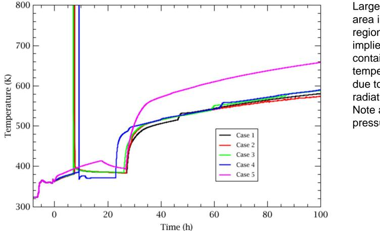
Large spreading area in floor region (Case 5) implies higher containment temperature due to heat radiation Note also higher pressure
