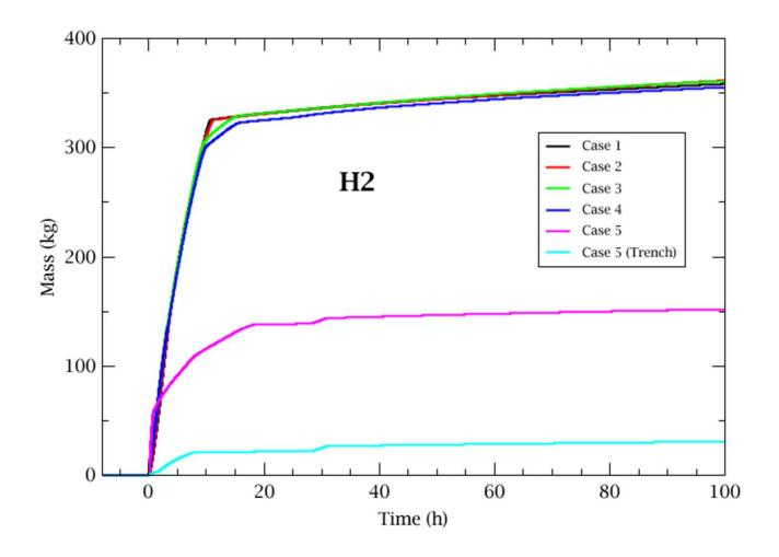
Hydrogen produced in "small trench" is only 20 % of total Hydrogen produced from MCCI
